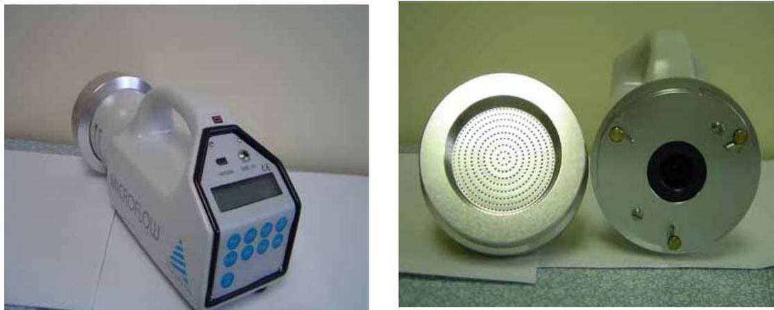
*Figure 3.* The Microflow, single-stage sampler and perforated head are shown.
