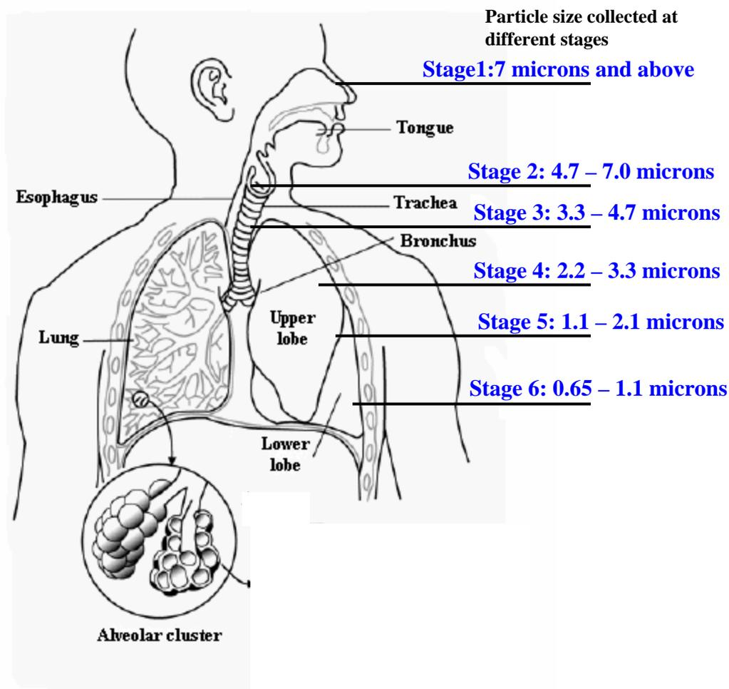
*Figure 5.* Andersen's sampler, a comparison with human respiratory tract, with diagram of human respiratory system from [http://www.asosh.org/Programmes/SORDSA/\\_derived/Crystalline\\_silica.htm\\_txt\\_Lung.gif](http://www.asosh.org/Programmes/SORDSA/_derived/Crystalline_silica.htm_txt_Lung.gif)
