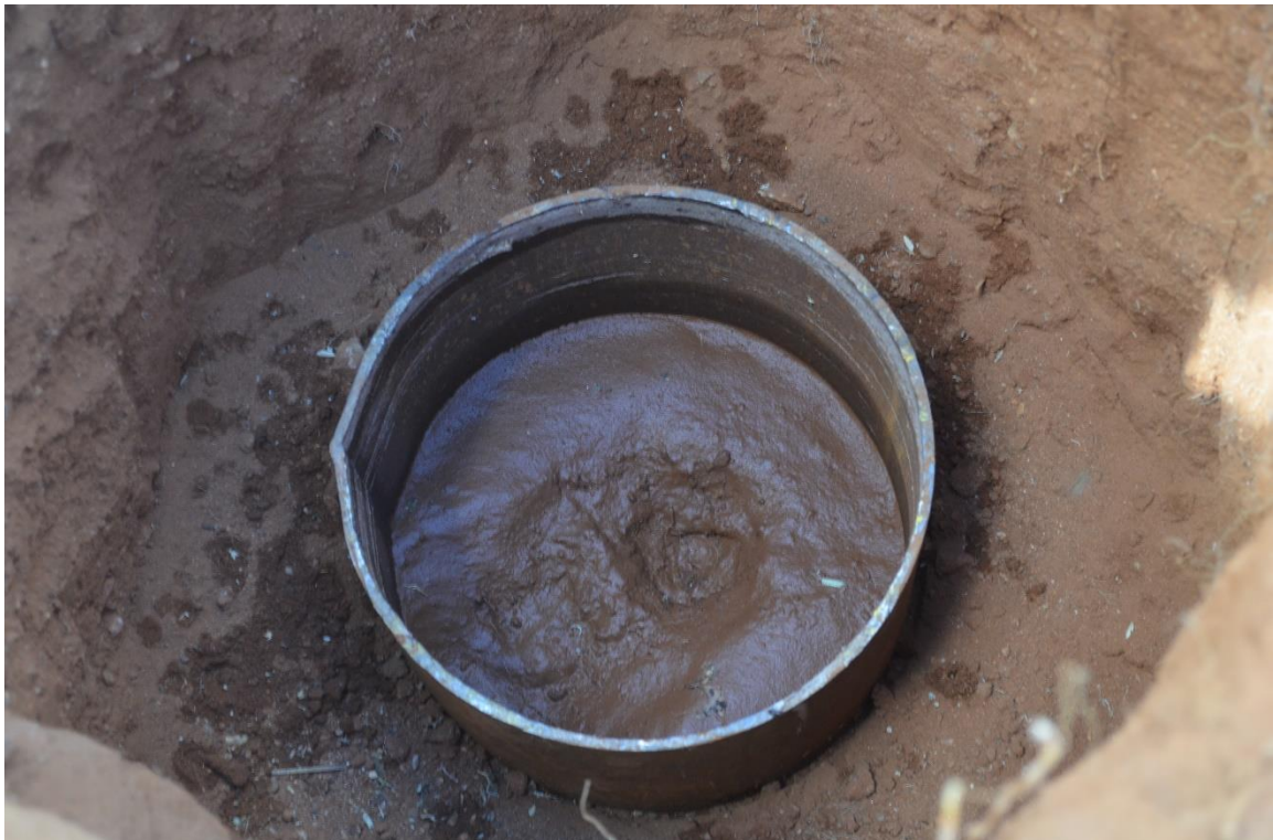
Figure 2: Sinkhole of soil after Ring Test
