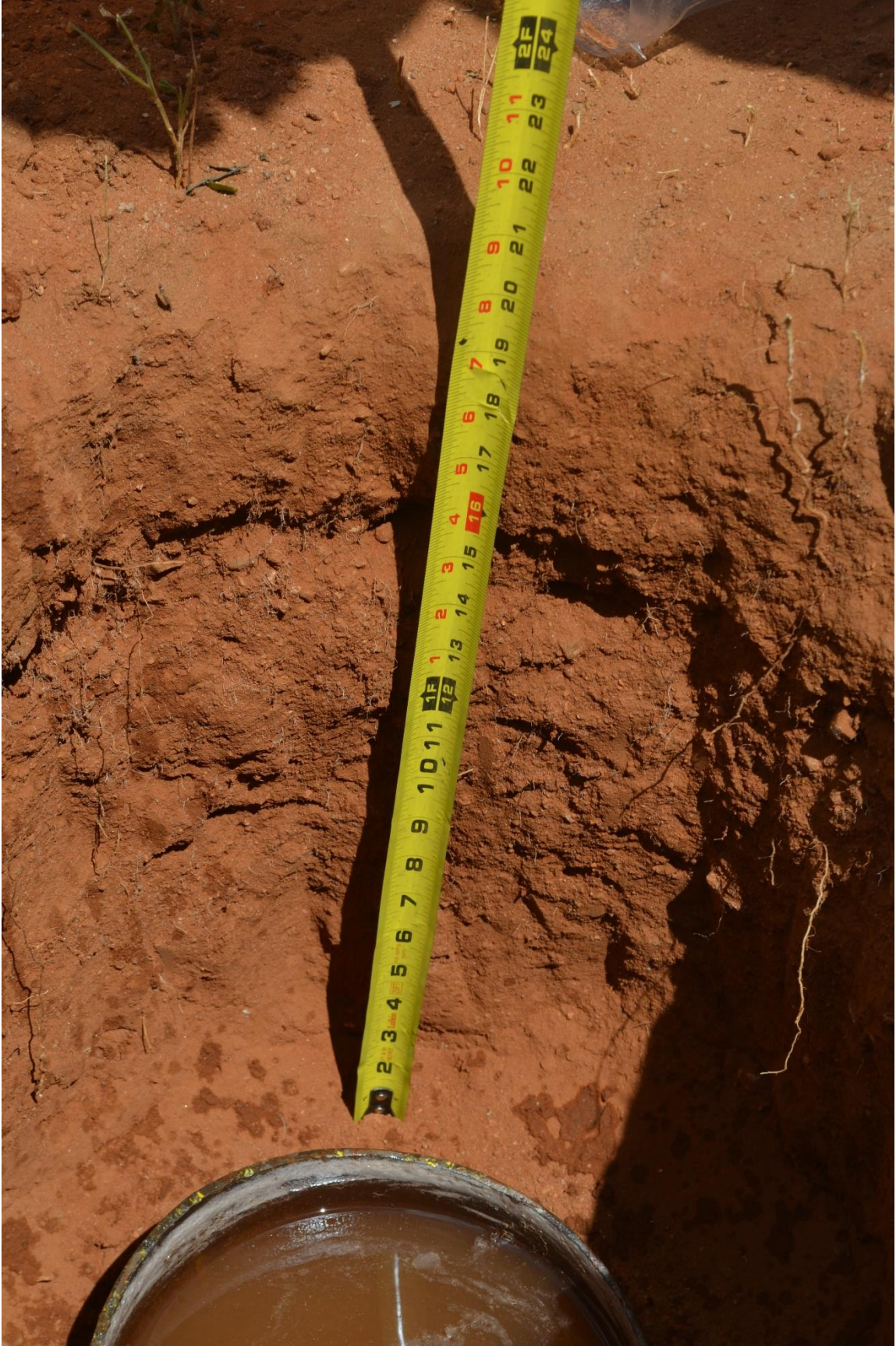
Figure 3: Soil Structure of Test 1
