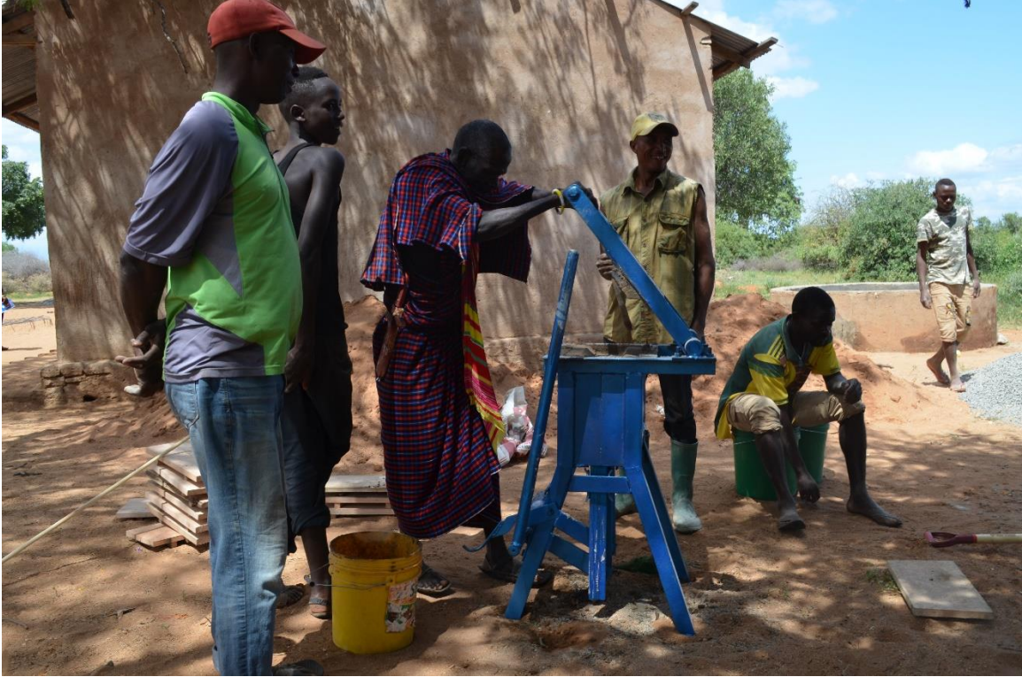
Figure 43: Block maker in use
