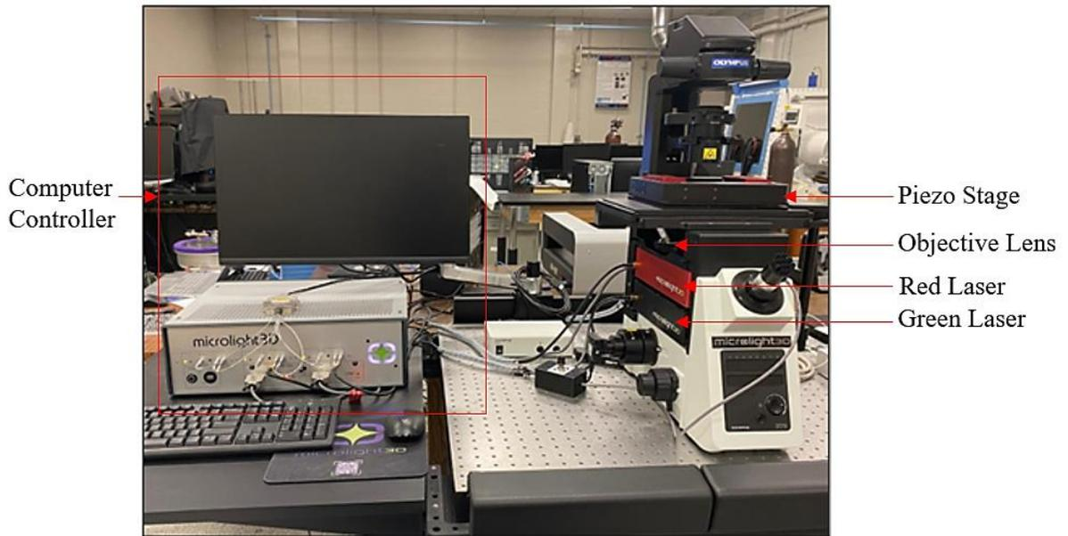
**Figure 3. 7:** Shows complete setup of the 2PP machine during fabrication in the Lab
