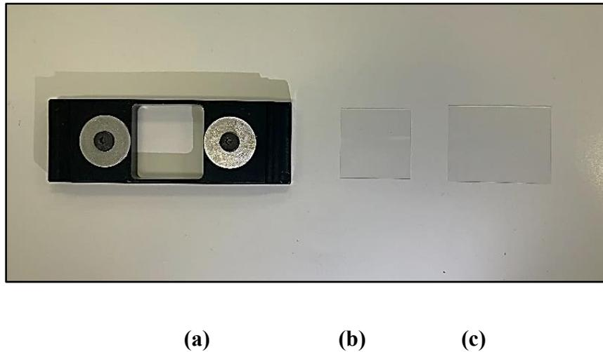
**Figure 3. 5:** (a) Sample holder, (b) Base coverslip (24x24mm), (c) Top coverslip (24x32 mm).
