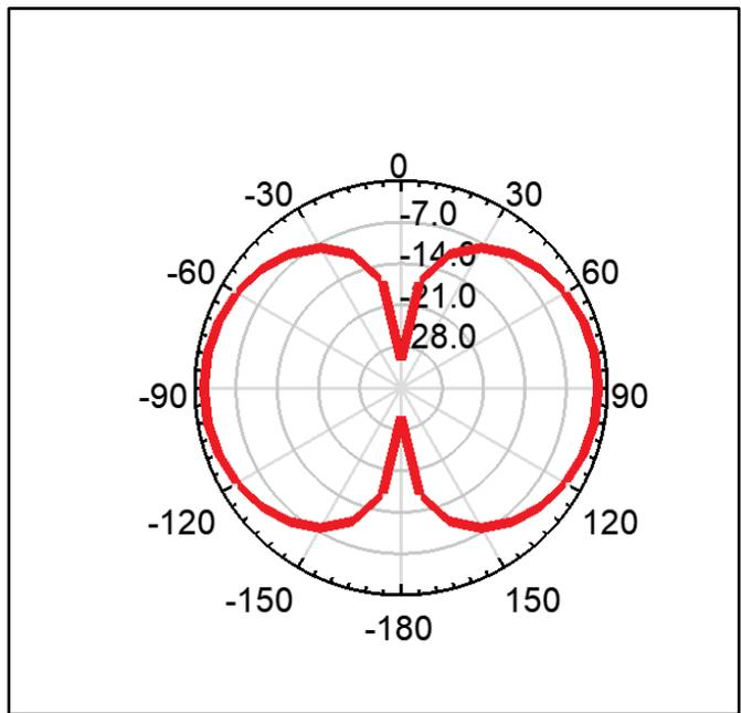
Figure 4. 3: Demonstrates the radiation pattern of the monopole THz antenna at 0.11 THz.
