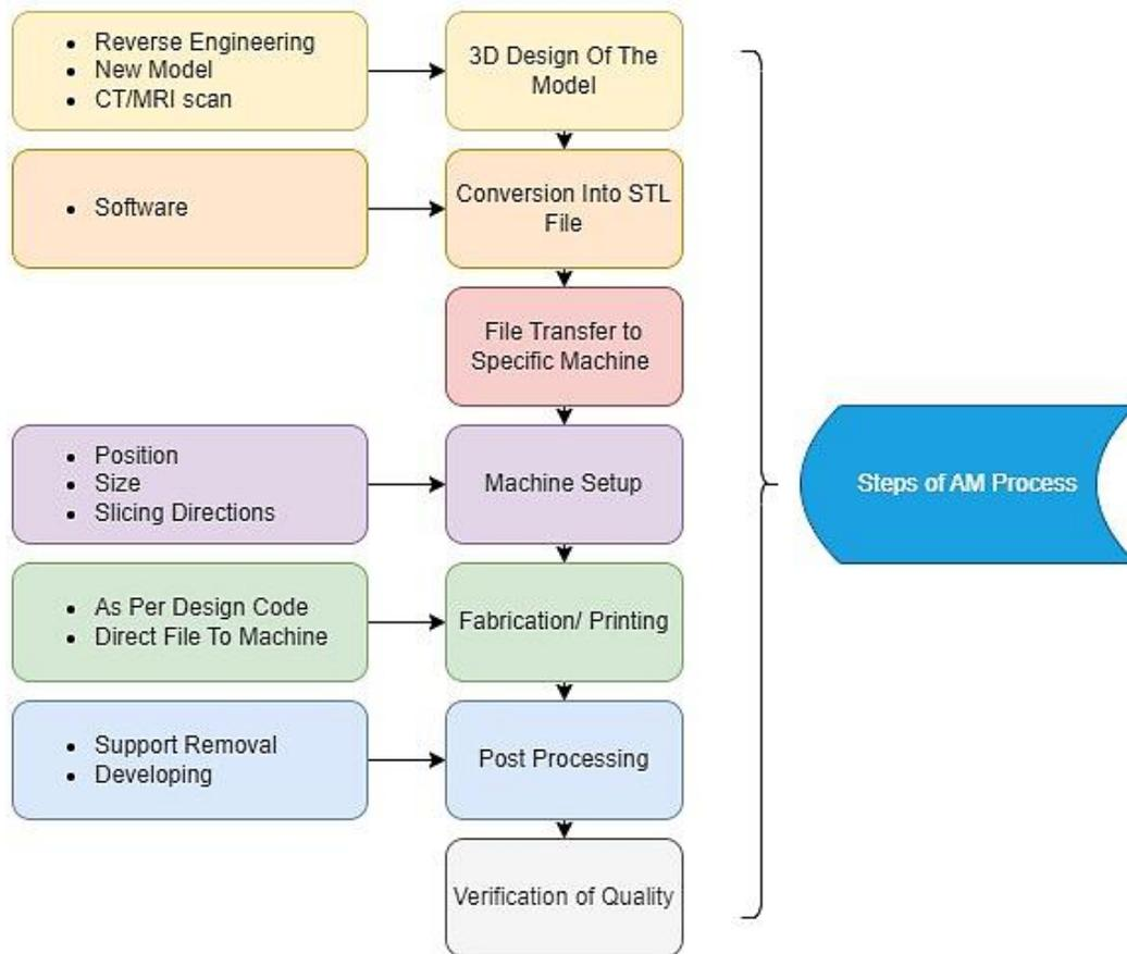
**Figure 2. 1:** Different steps of AM process.
