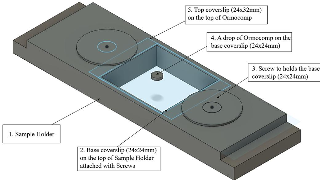
**Figure 3. 4:** Graphical representation of the complete setup of sample preparation
