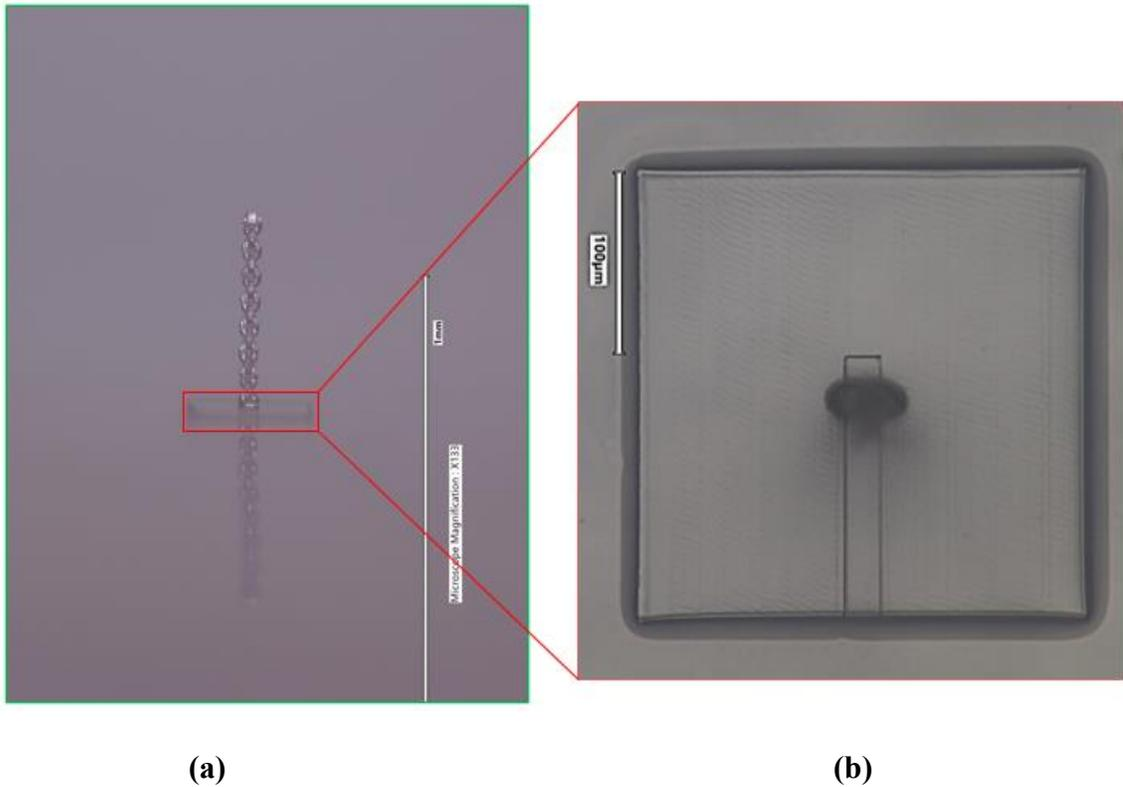
**Figure 4. 5:** Picture of (a) Chain, (b) Substrate and feed line from Keyence Microscope.
