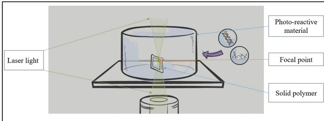
**Figure 2. 4:** Two photon polymerization technique [54]
