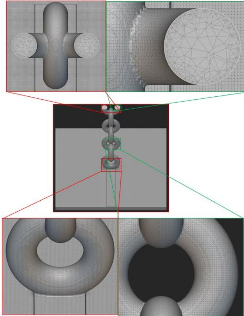
**Figure 3. 3:** Section cut view of the designed THz antenna in nTopology with inside and outside mesh
