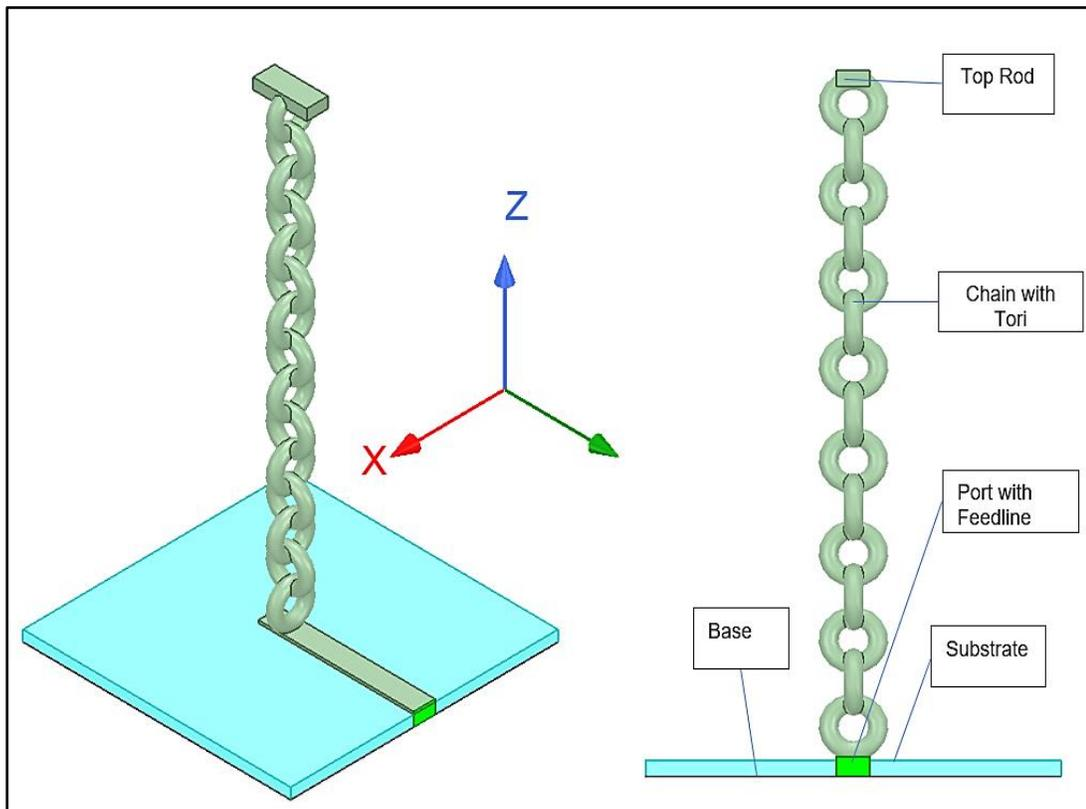
**Figure 3. 2:** Graphical representation (Left) and different components (Right) of THz monopole antenna from HFSS.
