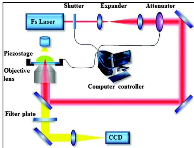
Figure 2. 2: A typical experimental setup of TPP[48]
