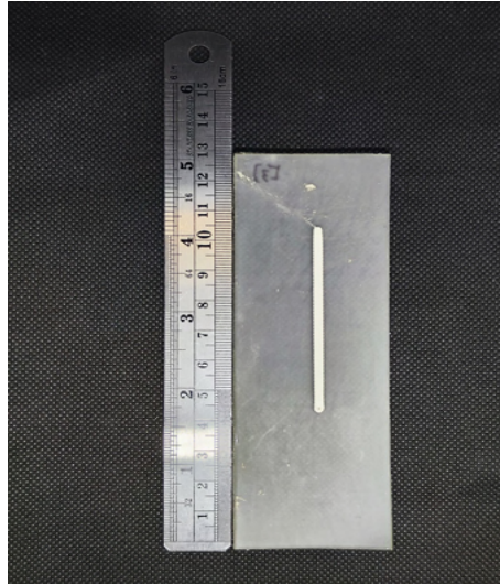
Figure 3.19. Printed flexible platform and conductive line for the adhesion test.
