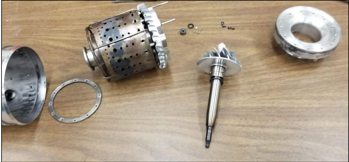
Figure 2-6: Disassembled Engine with Removed Compressor
