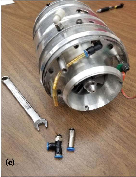
Figure 2-2: Removal of Sensors
