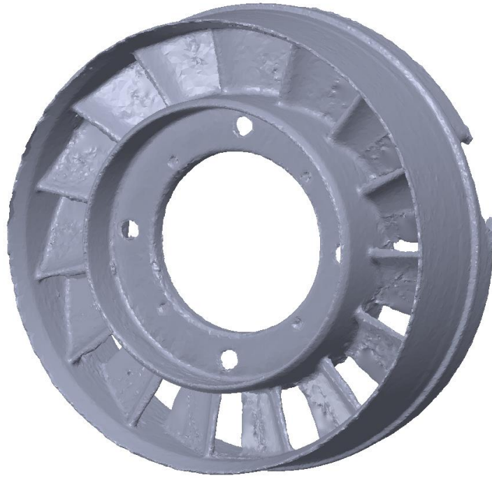
Figure 5-8: Turbine Stator Scan
