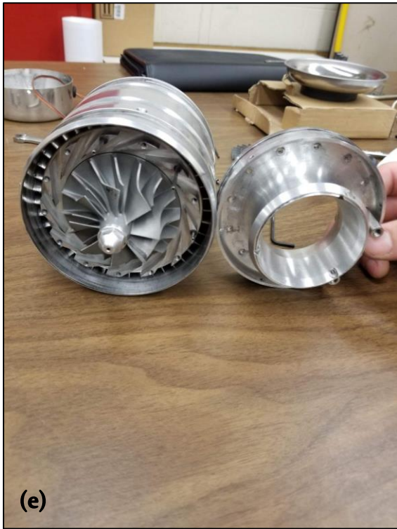
Figure 2-3: Exposed Compressor and Diffuser
