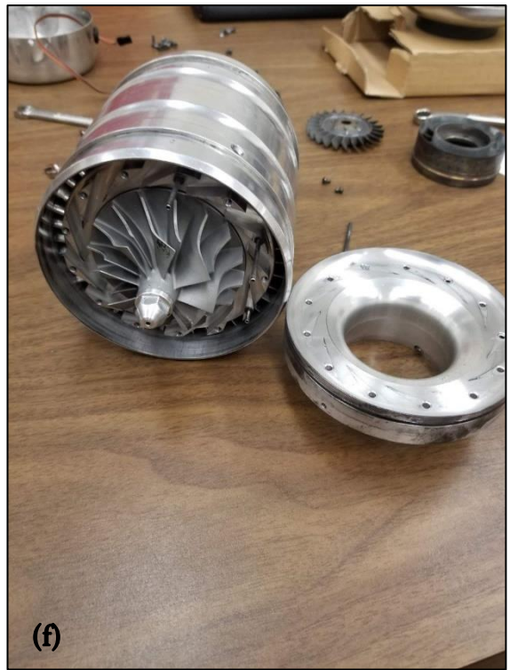
Figure 2-3: Exposed Compressor and Diffuser
