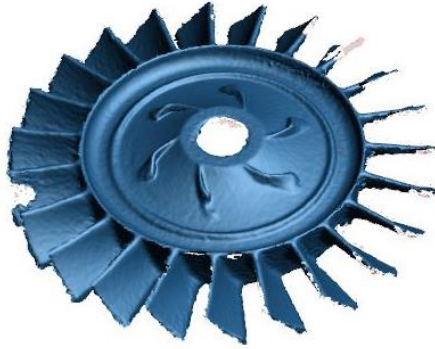
Figure 2-9: Cleaned Turbine Rotor Model
