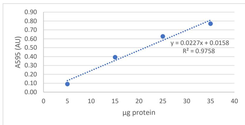
**Figure 6:** Bradford assay standard curve of absorbance at 595 nm verses micrograms of protein (BSA).
