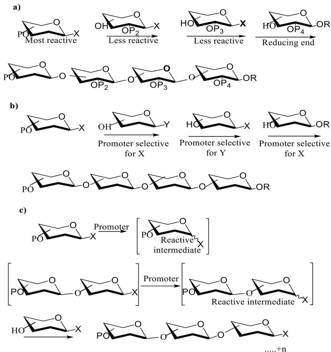
**Figure 2:** Example of one pot synthesis. PO, OH and O between C3 and C4 means they can be on either C3 or C4; P and R represent protecting groups. a) One pot synthesis based on chemo selective strategy; b) Orthogonal strategy; and c) Pre-activation strategy.<sup>47 48</sup>
