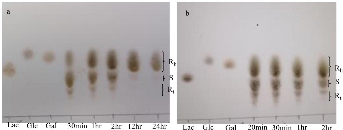
**Figure 8:** TLC analysis of the reactions using enzymes immobilized on a silica-chitosan support.  $R_h$  - hydrolysis products,  $R_t$  - transglycosylation products, S - substrate, Lac - lactose, Glc - glucose, and Gal - galactose. a) immobilized  $\beta$ -galactosidase enzyme from *Aspergillus oryzae*; b) immobilized lactase
