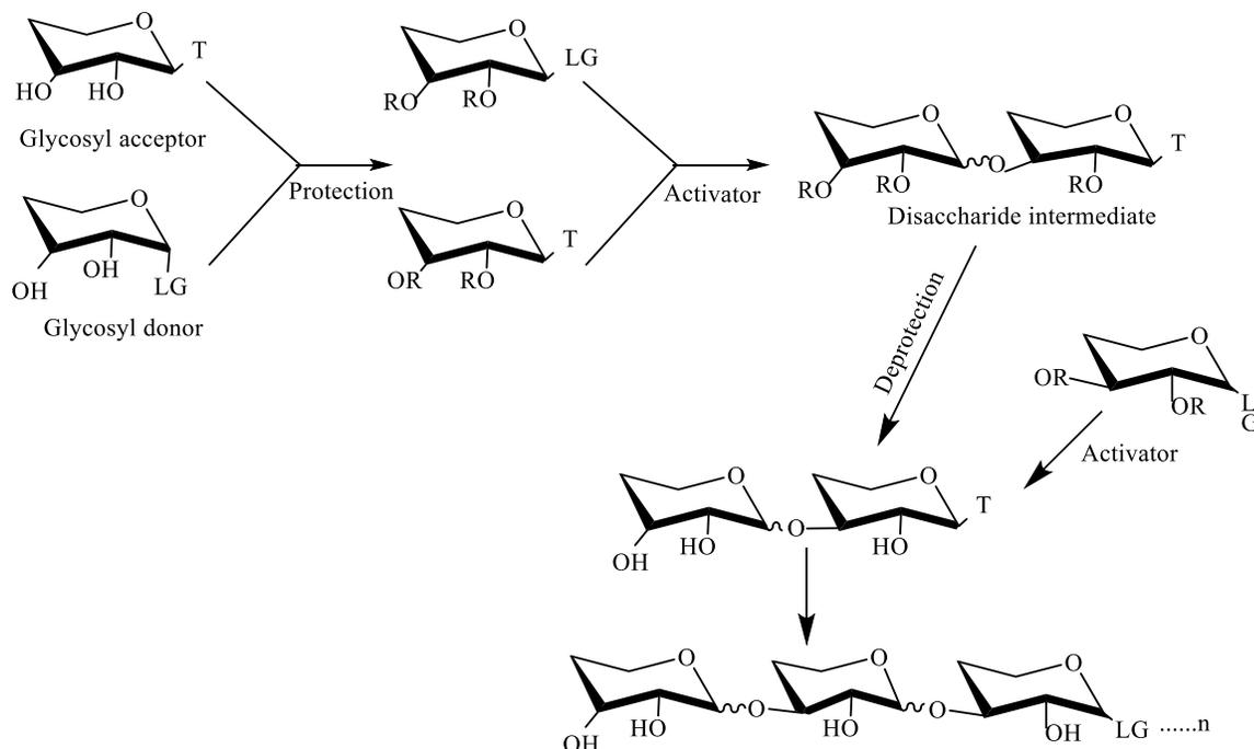
**Figure 1:** Typical chemical synthesis scheme for oligosaccharides where R represents the protecting groups, LG represents the leaving group, and T is a temporary group<sup>38, 48</sup>
