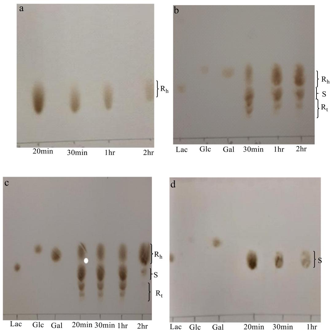
**Figure 10:** Effect of temperature on transglycosylation and hydrolysis reactions using immobilized lactase. Rh - hydrolysis products, Rt - transglycosylation products, S - substrate, Lac - lactose, Glc - glucose, and Gal - galactose. a) 25 °C, b) 50 °C, c) 60 °C , d) 75 °C.
