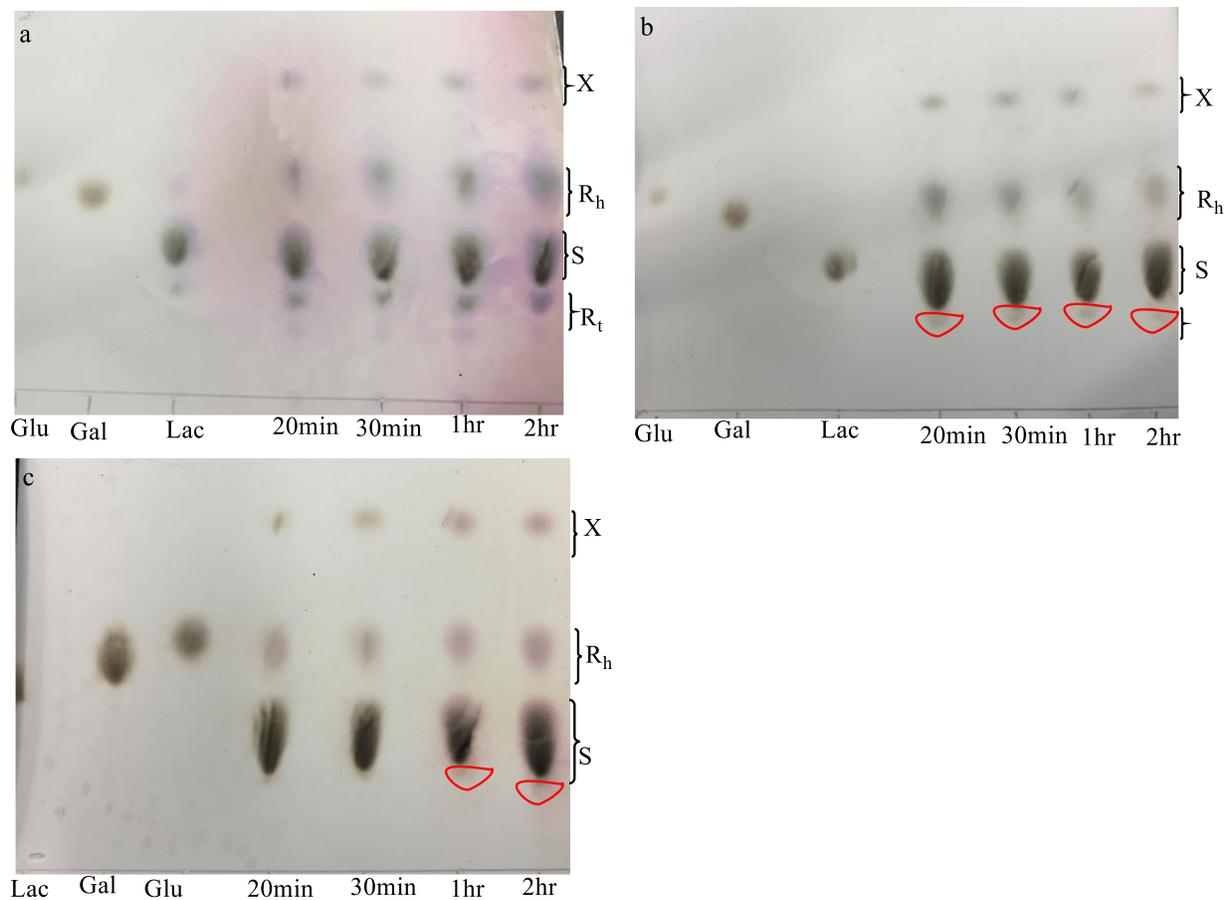
**Figure 14:** Effect of 1-butanol on transglycosylation and hydrolysis activity of immobilized lactase,  $R_h$  - hydrolysis products, X- unknown products,  $R_t$  - transglycosylation products, S- substrate, Lac - lactose, Glc - glucose, and Gal - galactose. a) the reaction in 15 % v/v 1-butanol, b) the reaction in 25% v/v 1-butanol, c) the reaction in 50% 1-butanol
