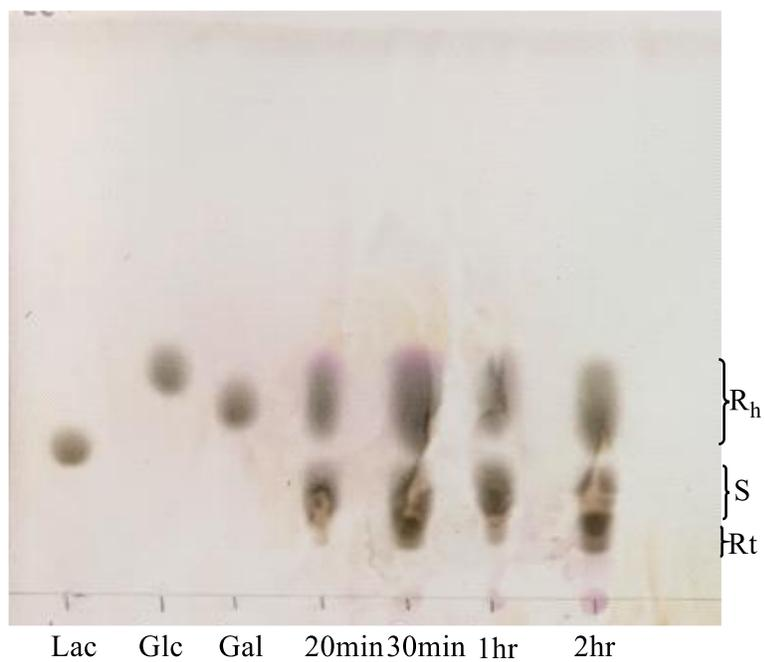
**Figure 26:** TLC analysis for products formed from 400 mM lactose using free *Enterobacter*  $\beta$ -galactosidase. S- substrate, Glc - glucose, Gal – galactose, Lac – lactose;  $R_h$  - hydrolysis products; and  $R_t$  - transglycosylation products.
