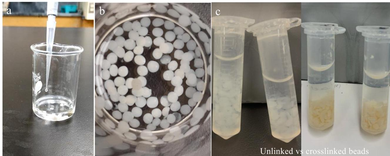
**Figure 5:** Chitosan-silica beads (ChtS) **a)** making ChtS beads, **b)** ChtS beads **c)** un-linked ChtS beads (left) versus ChtS beads cross-linked with glutaraldehyde (right).
