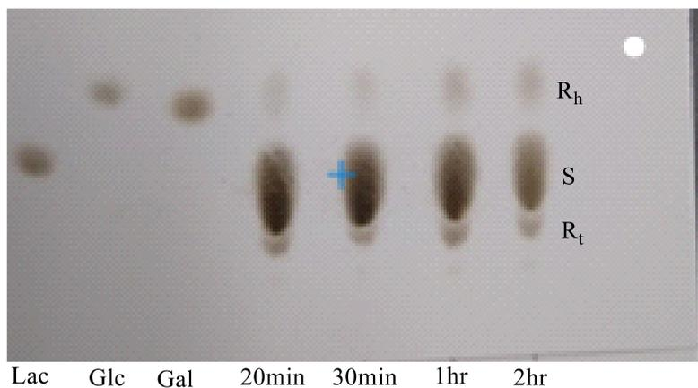
**Figure 7:** TLC analysis for products formed from 400 mM lactose using free enzyme  $\beta$ -galactosidase from *Aspergillus oryzae*. S - substrate, Glc - glucose, Gal – galactose, Lac – lactose, R<sub>h</sub> - hydrolysis products, and R<sub>t</sub> - transglycosylation products.
