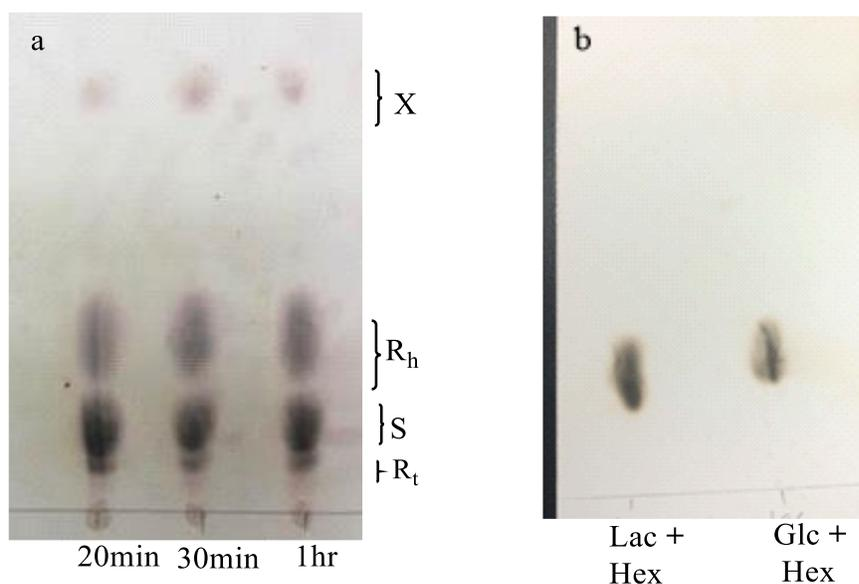
**Figure 15:** a) Transglycosylation and hydrolysis activity of immobilized lactase run in a hexanol/buffer two-phase system.  $R_h$  - hydrolysis products, X - unknown products,  $R_t$  - transglycosylation products, S - substrate, Lac - lactose, Glc - glucose, and Gal – galactose, b) Reaction between 1-hexanol and sugar (lactose or glucose).
