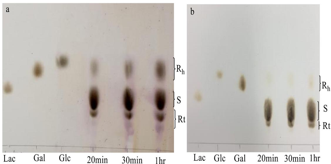
**Figure 16:** Time course of transglycosylation and hydrolysis catalyzed by immobilized lactase in presence of phenols in the reaction media, R<sub>h</sub> - hydrolysis products, R<sub>t</sub> - transglycosylation products, S - substrate, Lac - lactose, Glc - glucose, and Gal - galactose. a) 0.1 M 4-nitrophenol and b) 0.1 M phenol.
