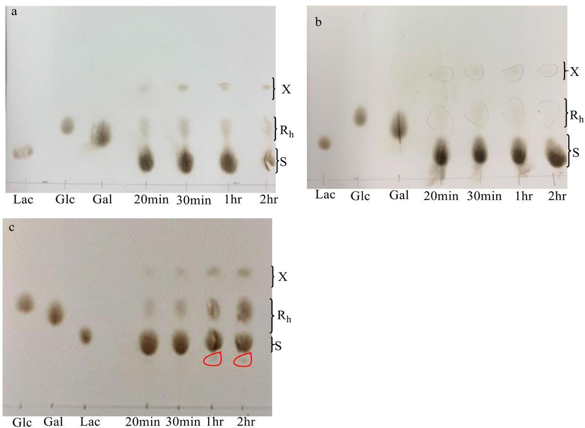
**Figure 13:** Effect of 2-propanol on transglycosylation activity of immobilized lactase  $R_h$  - hydrolysis products, X - unknown products,  $R_s$  - transglycosylation products, S - substrate, Lac - lactose, Glc - glucose, and Gal - galactose. a) 15% v/v 2-propanol in the reaction, b) 25% v/v 2-propanol in the reaction, c) 50% v/v 2-propanol in the reaction mixture
