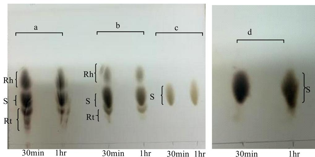
**Figure 18:** Reusability test of immobilized lactase at 60 °C. The immobilized enzyme lactase was used consecutively for four cycles at 60 °C: Rh - hydrolysis products, Rt - transglycosylation products, S - substrate, Lac - lactose, Glc - glucose, and Gal - galactose. a) trial 1, b) trial 2, c) trial 3, and d) trial 4.
