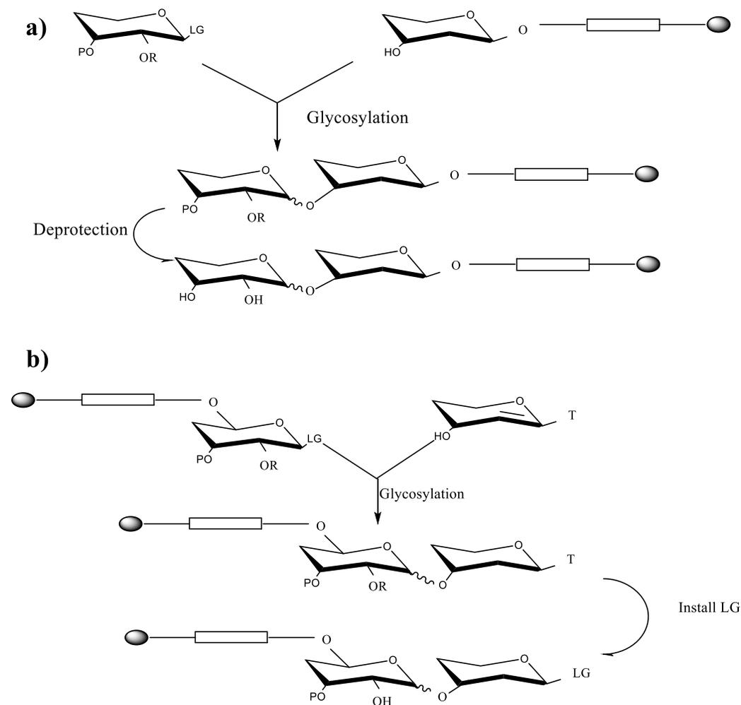
**Figure 3:** Solid support oligosaccharide synthesis. R and P - protecting groups, LG - leaving group, and T - temporary group. a) Solid support oligosaccharide synthesis based on acceptor-bound approach; b) Solid support oligosaccharide synthesis based on donor-bound approach.<sup>47</sup>
