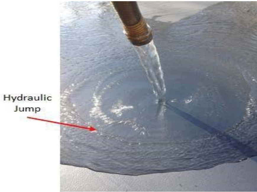
Figure 5: Hydraulic jump caused by a regular household hose.
