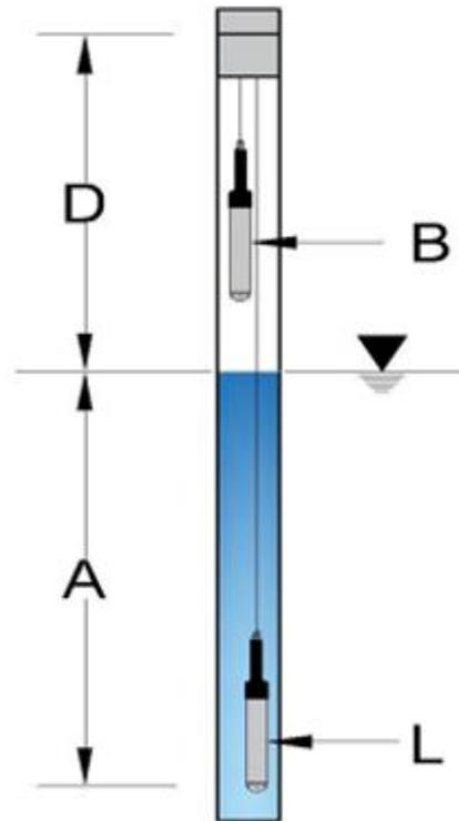
Figure 2-10: Working principle of Levelogger and Barologger
