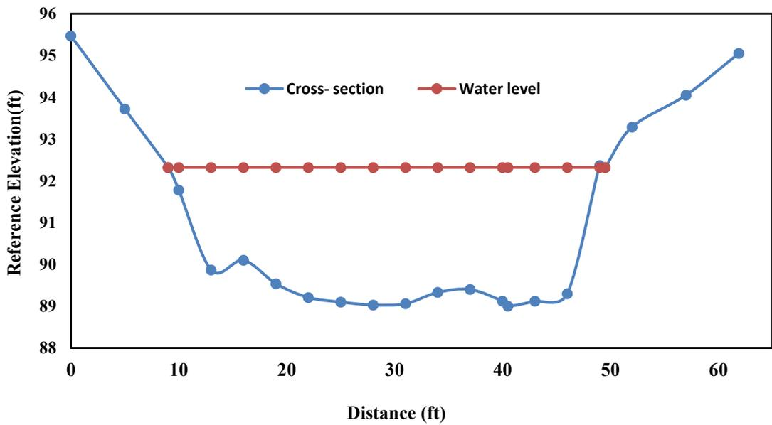
Figure 2-8: Marsh Creek cross-section at flow monitoring site
