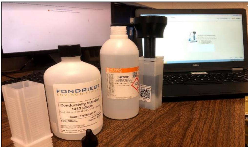
Figure 2-3: Calibration of Levellogger before instrument installation
