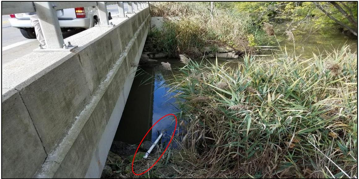
Figure 2-6: Levelogger instrument setup on the downstream side of Marsh Creek Bridge on Lake Shore Boulevard
