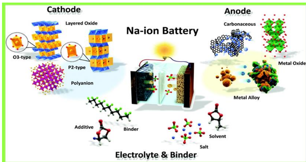
Figure 1: Schematics of working principle of a Sodium-Ion Battery (14)
