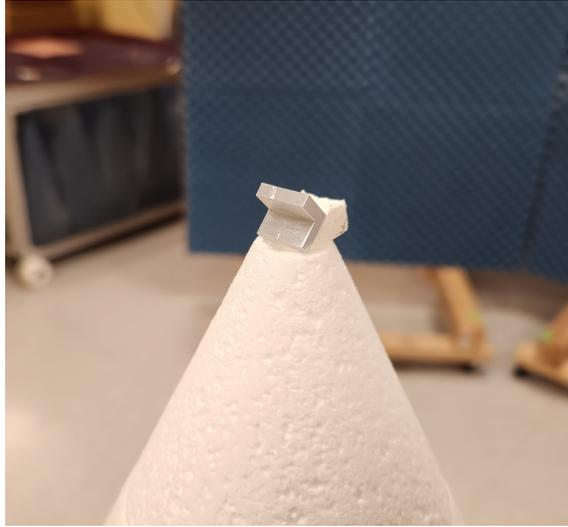
Figure 3.18: Scale model dihedral mounted on foam pedestal.
