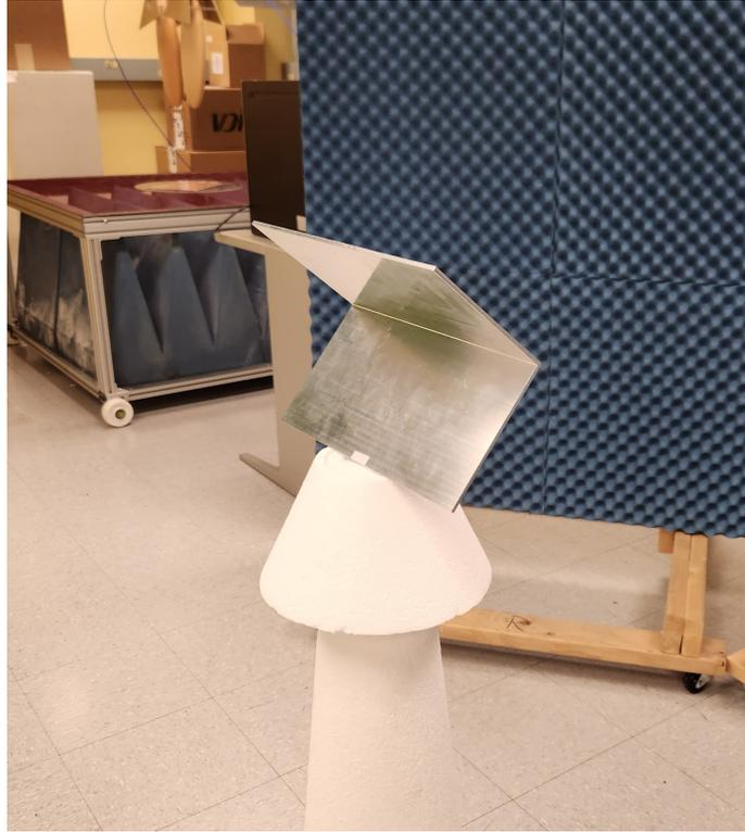
Figure 3.19: Ka-band dihedral mounted on foam pedestal.
