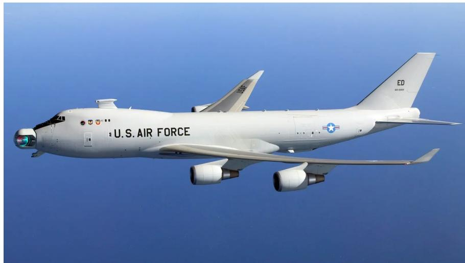
Figure 1: Boeing YAL-1 Airborne Laser Testbed in flight<sup>6</sup>
