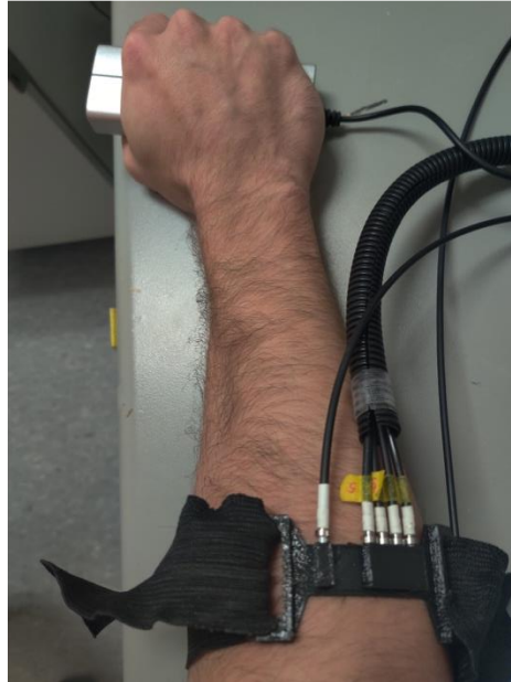
FIGURE 5-2 SETUP POSITION OF AN EXAMPLE SUBJECT FOR THE GRIP STRENGTH AND BLOODFLOW MEASUREMENT EXPERIMENT. THE GRIP FORCE DYNAMOMETER IS GRIPPED IN THE RIGHT (DOMINANT) HAND, AND THE DCS PROBE IS POSITIONED ON THE FOREARM, SECURED BY A FLEXIBLE NYLON BAND.
