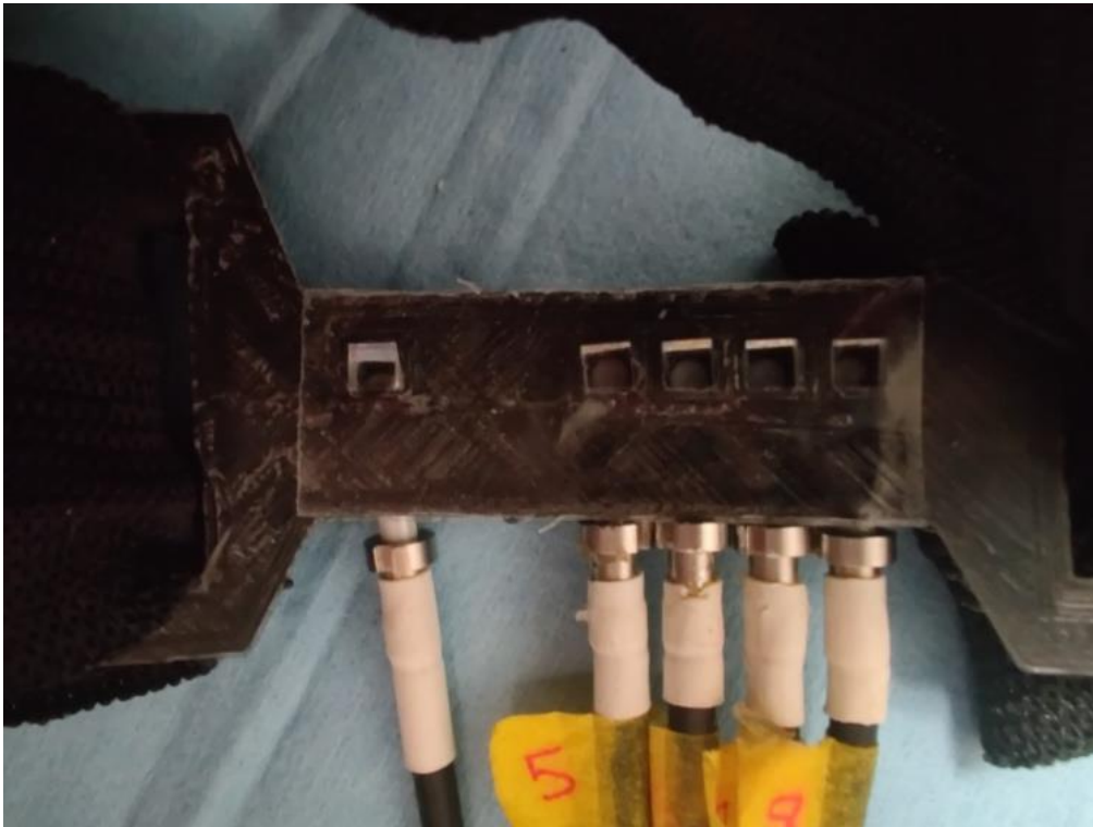
FIGURE 5-1 DCS IMAGING PROBE USED TO MEASURE BLOOD FLOW DURING GRIP FORCE TASK. OPTICAL FIBERS ARE USED FOR LIGHT TRANSPORT. FROM LEFT TO RIGHT; SOURCE FIBER, 1.5 CM DETECTOR, 2.0 CM DETECTOR, 2.5 CM DETECTOR, 3.0 CM DETECTOR.
