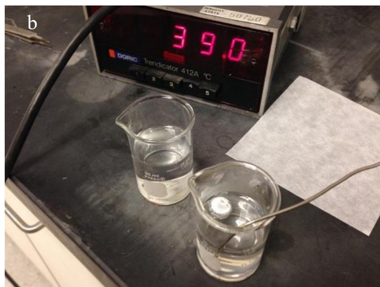
**Figure 6. 4 Composite response to temperature a)below LCST b) above LCST**
