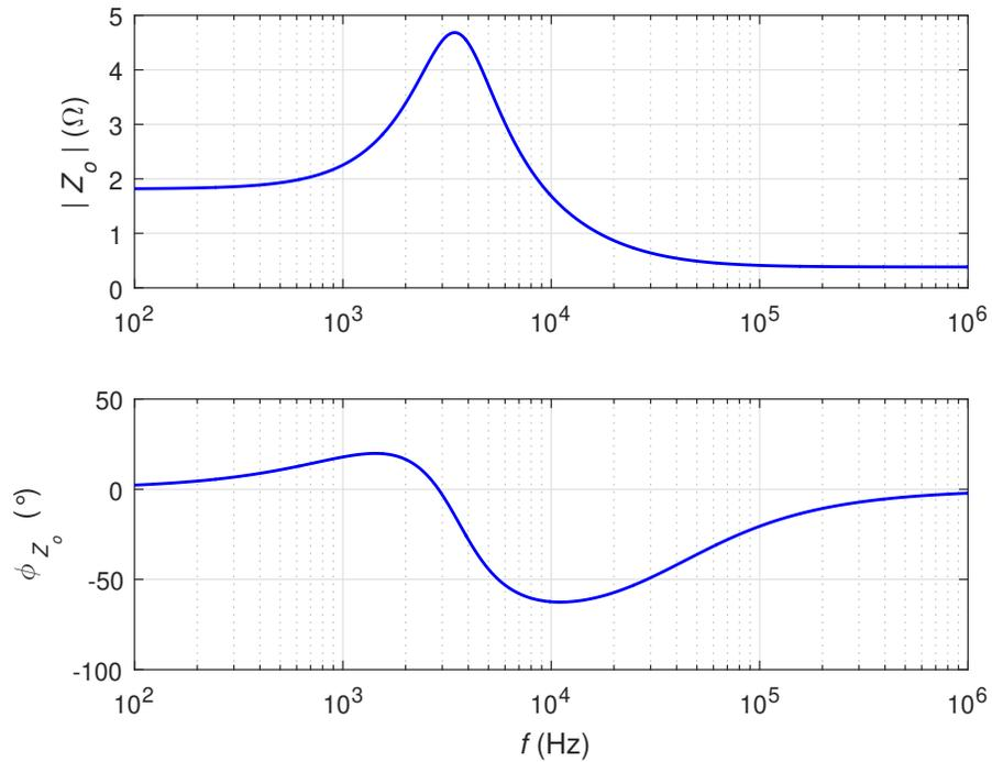
Figure 4.8: Calculated frequency response for output impedance transfer function.
