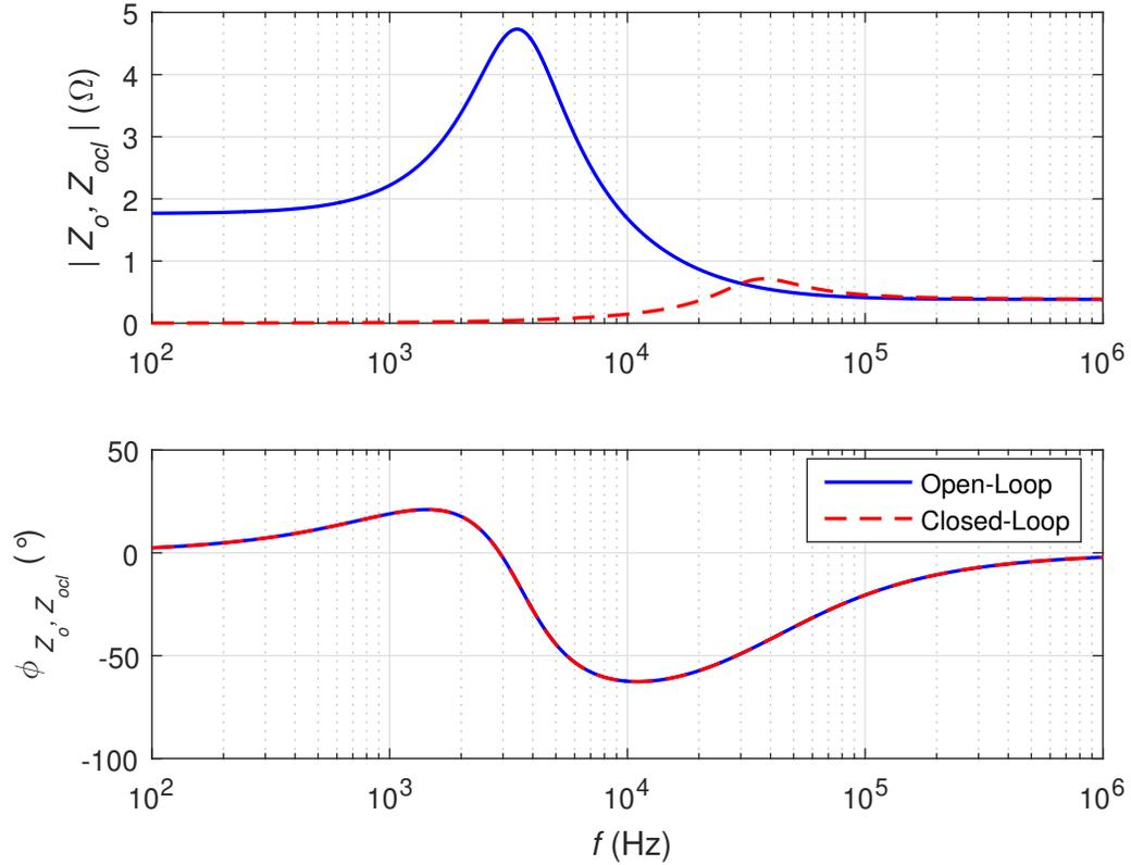
Figure 5.4: Calculated closed-loop output impedance frequency response, versus open-loop output impedance frequency response.
