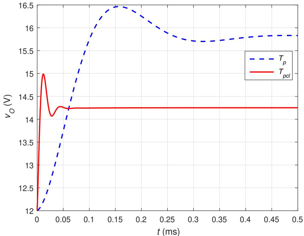
Figure 5.10: Calculated closed-loop control-to-output step response, versus open-loop control-to-output step response.
