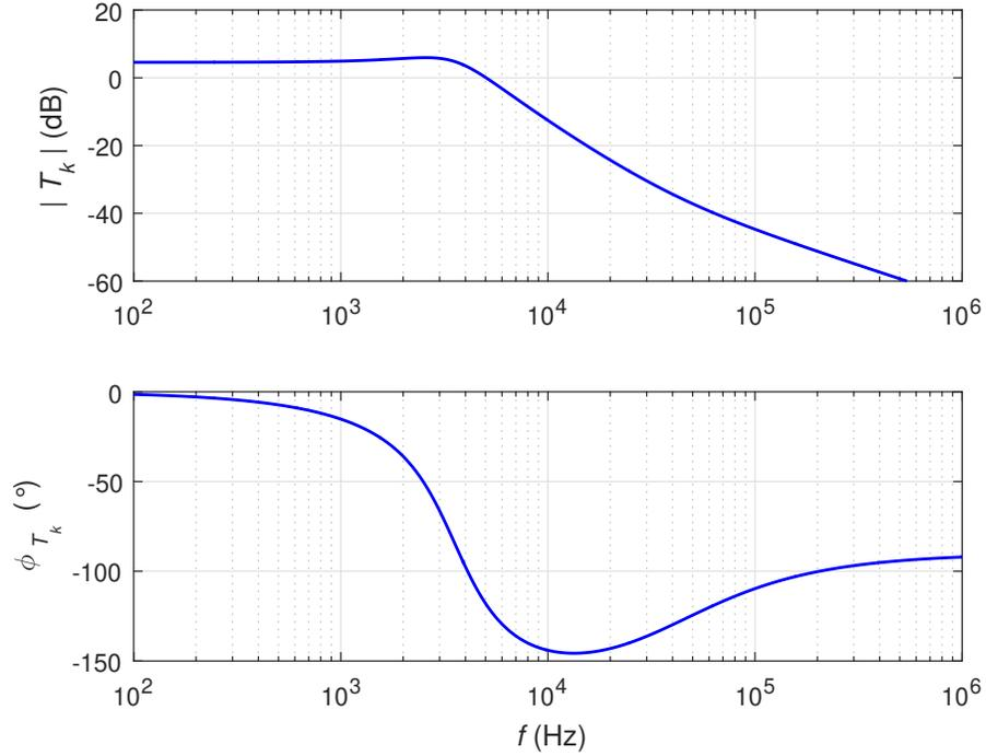
Figure 4.9: Calculated frequency response for the uncompensated system transfer function.
