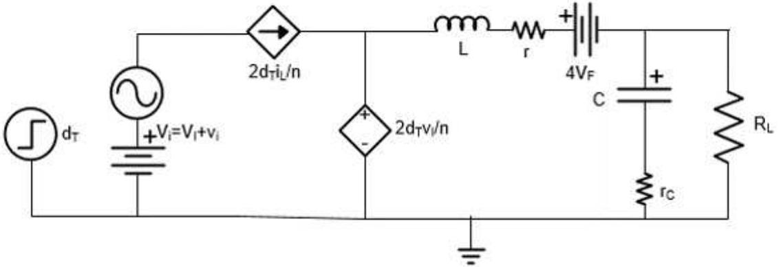
Figure 2.6: The reduced, averaged large-signal and small-signal model of the full-bridge DC/DC converter.
