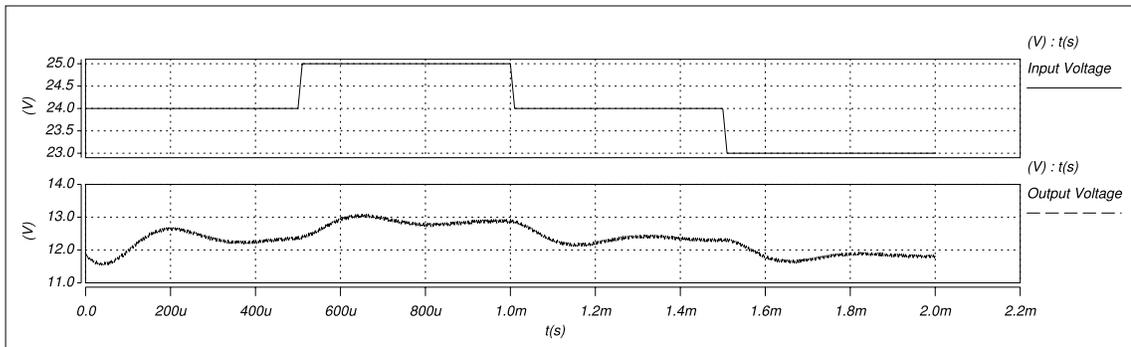
Figure 5.7: Simulated closed-loop audio susceptibility step response.
