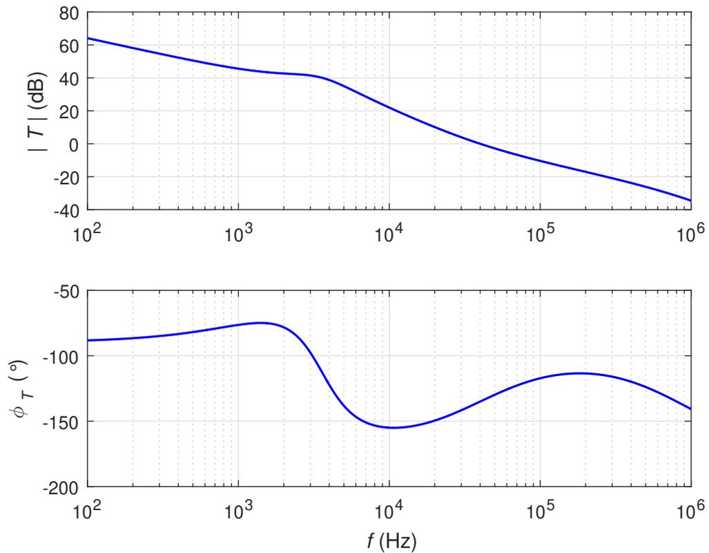
Figure 5.1: Calculated closed-loop system frequency response.
