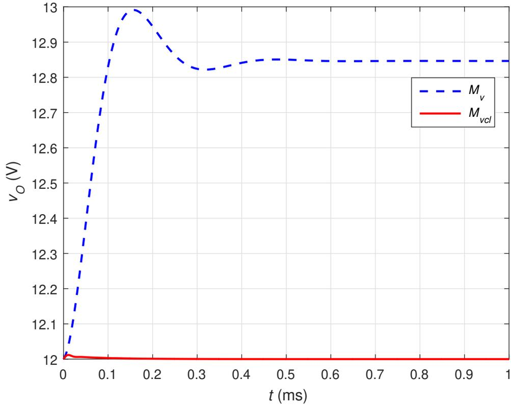
Figure 5.6: Calculated closed-loop input-to-output step response, versus open-loop input-to-output step response.
