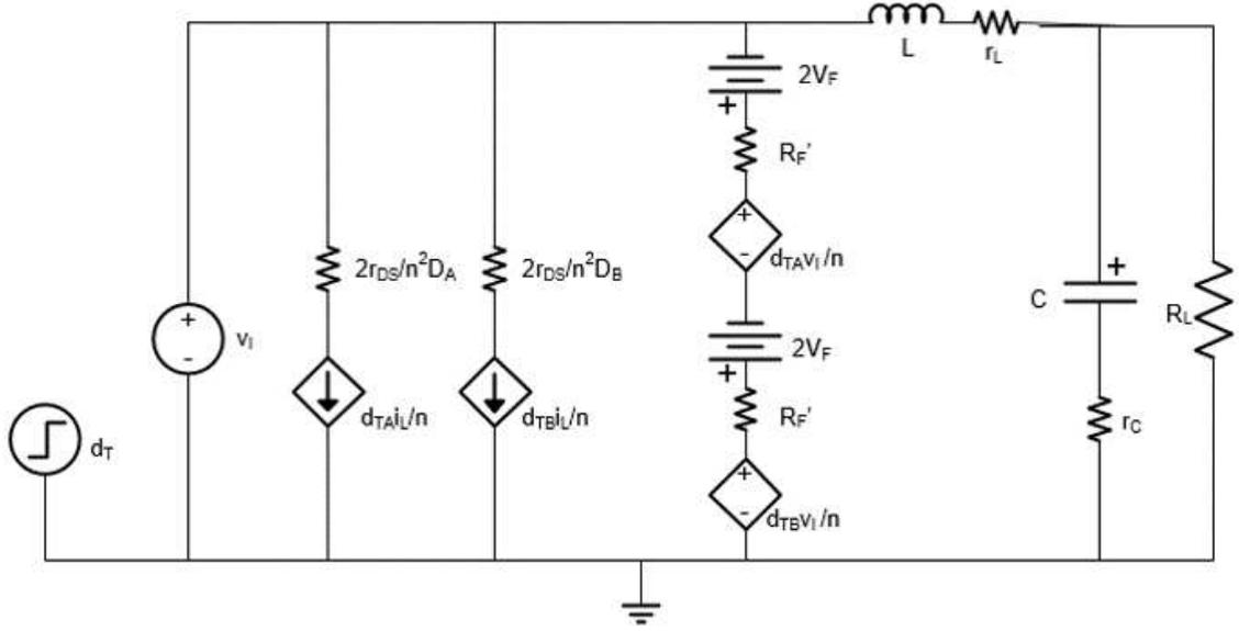
Figure 2.4: The partially reduced model of full-bridge DC/DC converter.
