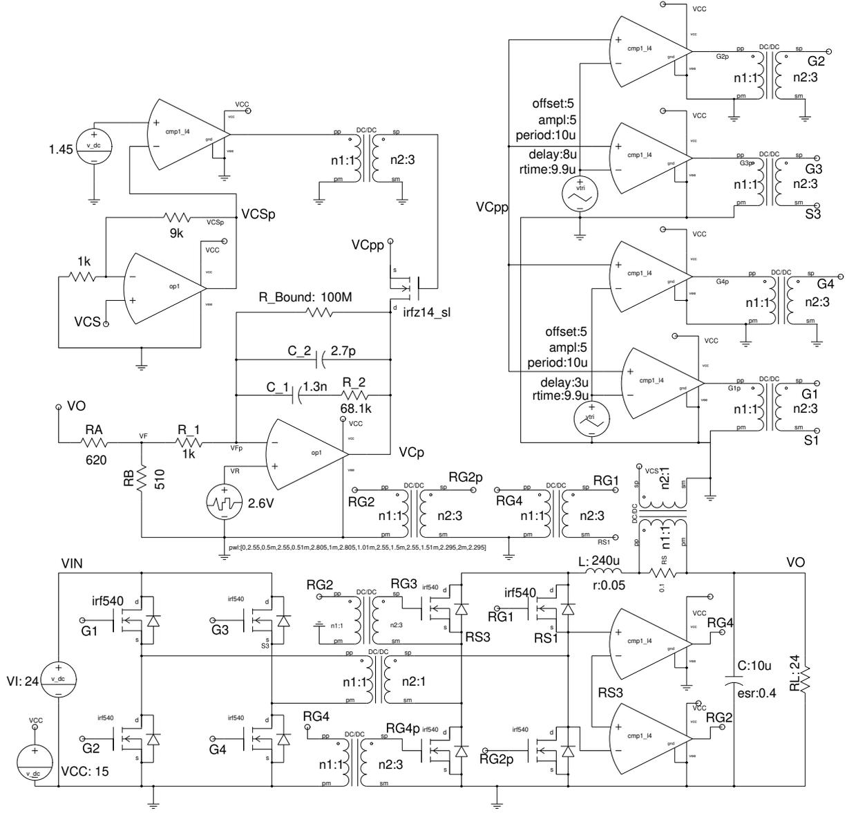
Figure 5.5: Simulated full-bridge DC/DC converter design [18]
