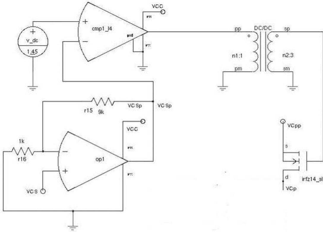
Figure 4.12: Active current-limiting circuit.
