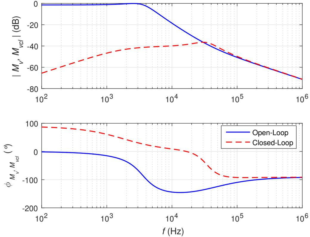
Figure 5.3: Calculated closed-loop input-to-output frequency response, versus open-loop input-to-output frequency response.
