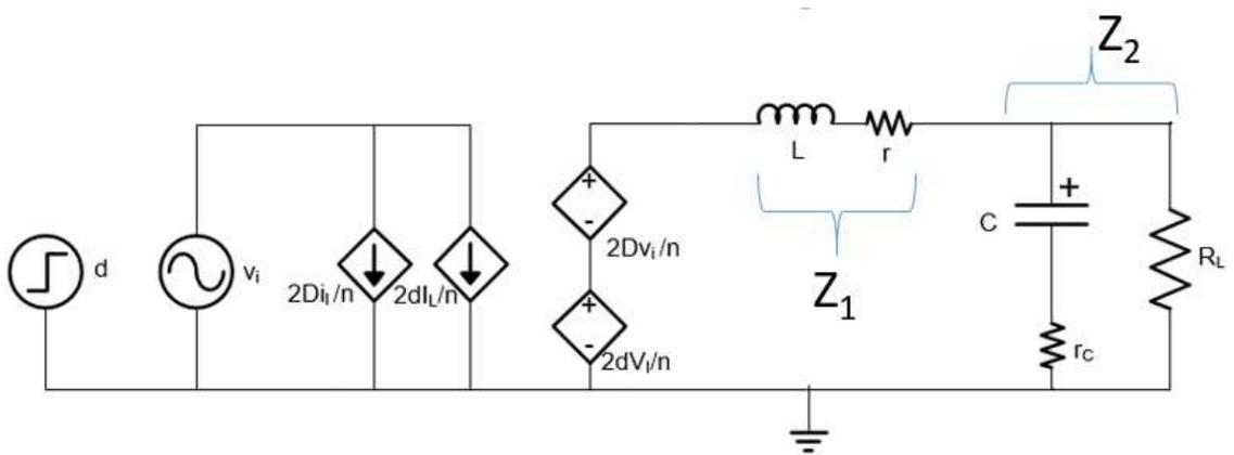
Figure 2.8: The reduced, averaged small-signal model of full-bridge DC/DC converter.
