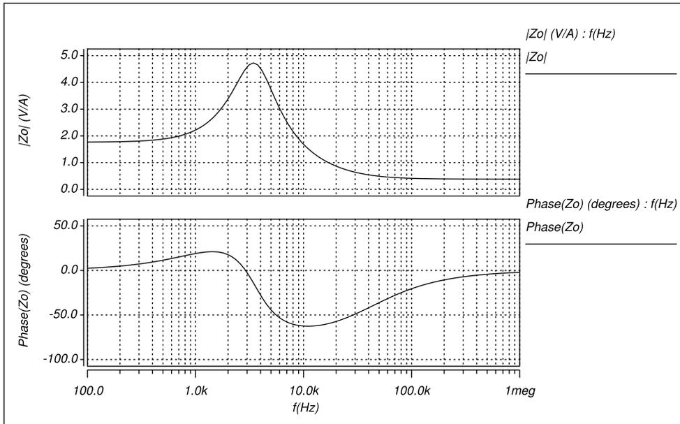
Figure 4.7: Simulated frequency response for output impedance transfer function.
