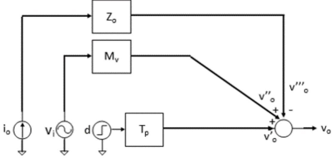
Figure 3.1: Block diagram of the small-signal model [1].
