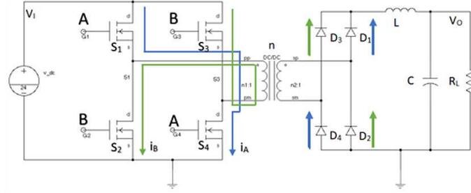
Figure 2.1: Basic circuit diagram of a full bridge DC/DC converter.
