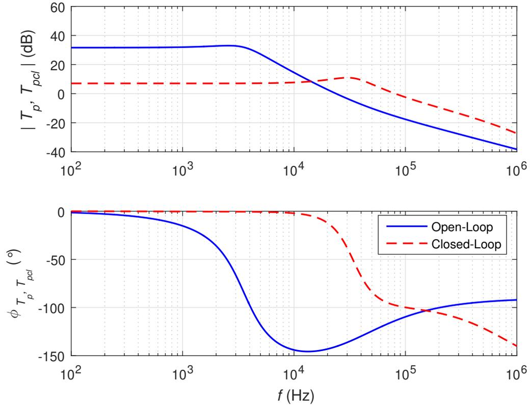
Figure 5.2: Calculated closed-loop control-to-output frequency response, versus open-loop control-to-output frequency response.
