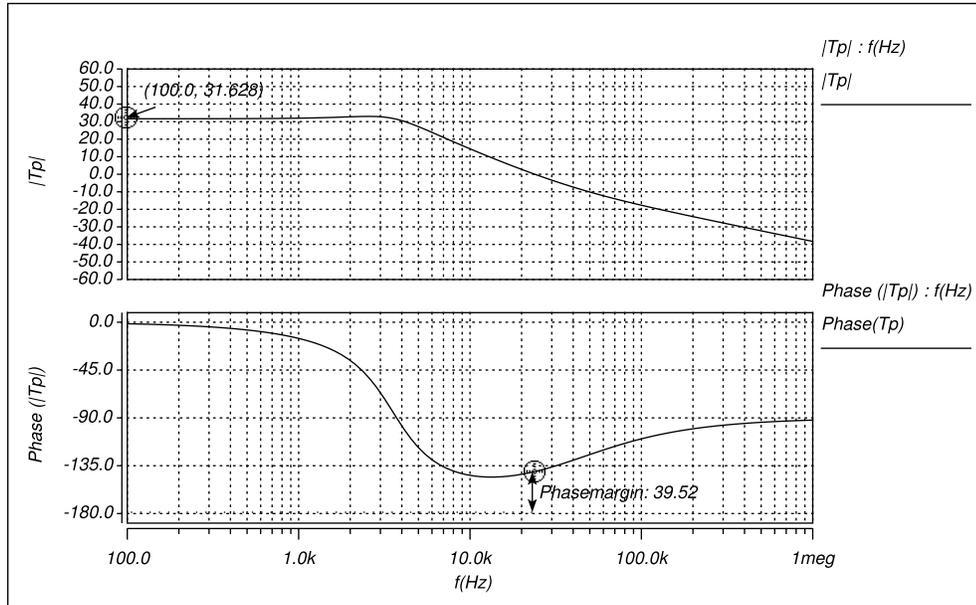
Figure 4.2: Simulated frequency response for control-to-output transfer function.
