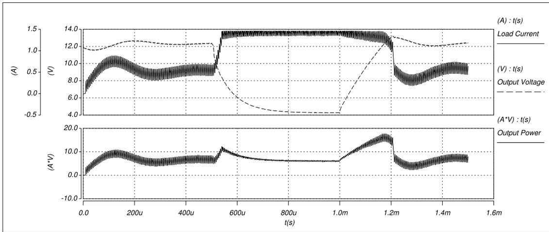
Figure 5.12: Simulated current limit results for an over-current condition in the full-bridge DC/DC converter.
