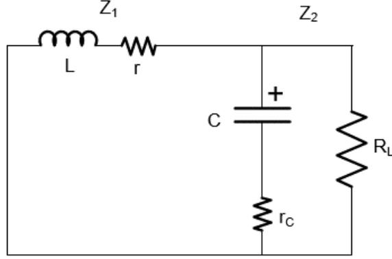
Figure 3.2: Output impedance analysis circuit.
