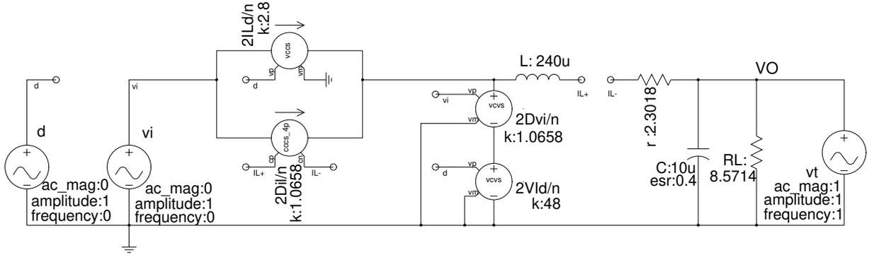
Figure 4.6: Simulated small-signal model for output impedance analysis.
