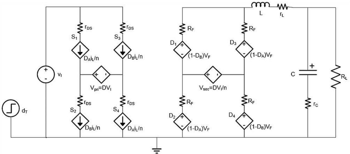
Figure 2.3: The unreduced model of full-bridge DC/DC converter.
