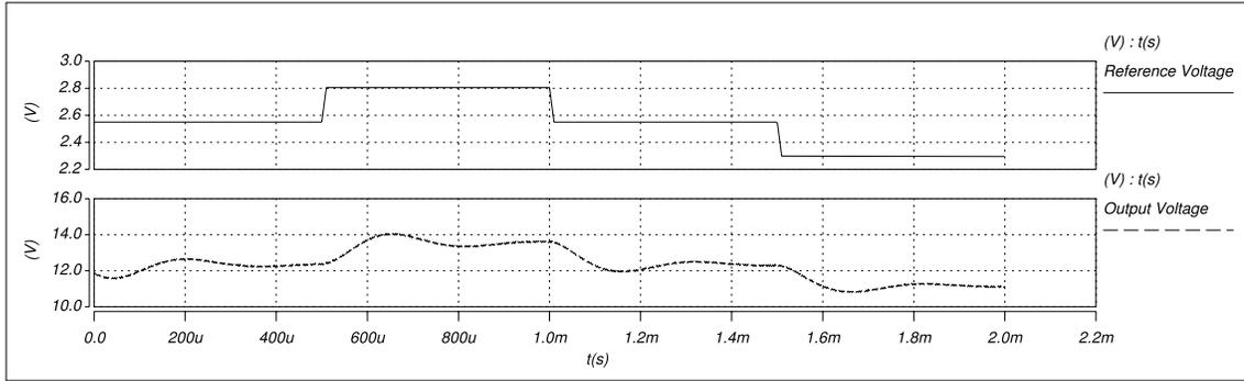
Figure 5.11: Simulated closed-loop control-to-output step response.
