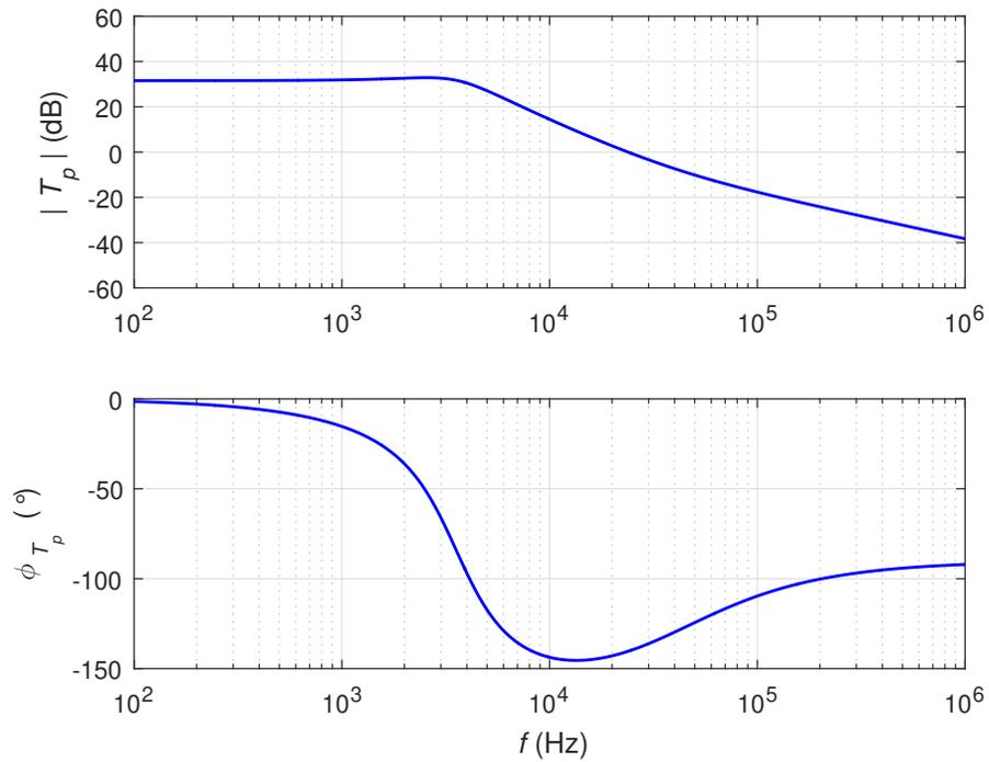
Figure 4.3: Calculated frequency response for control-to-output transfer function.
