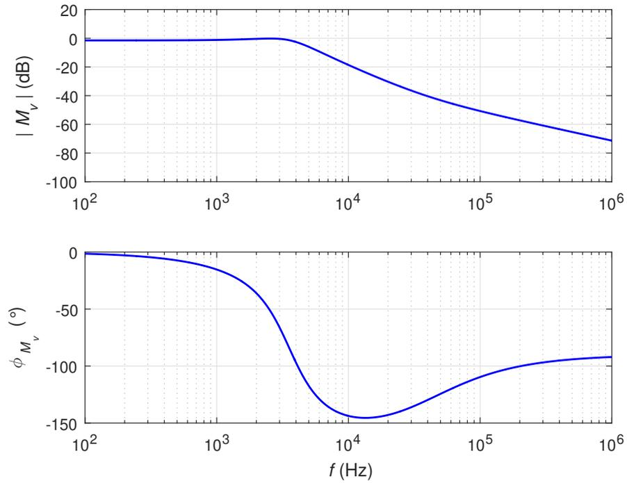
Figure 4.5: Calculated frequency response for input-to-output transfer function.
