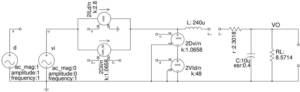
Figure 4.1: Simulated small-signal model for control-to-output analysis.
