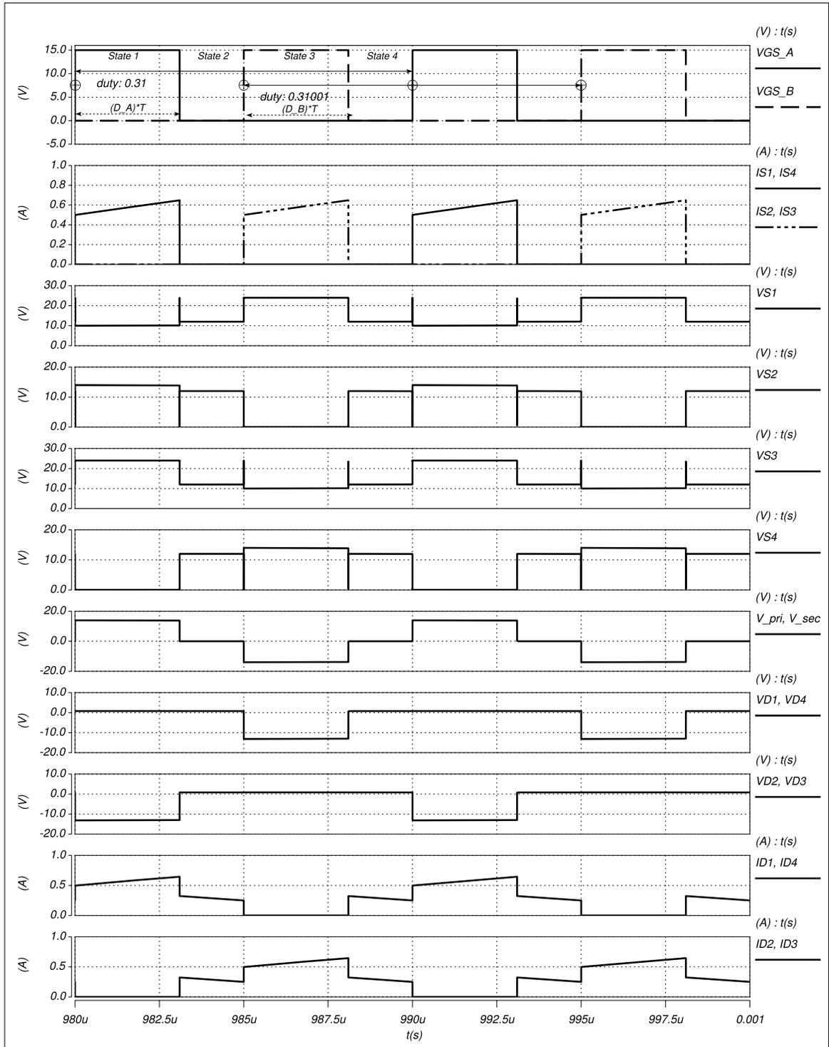
Figure 2.2: General waveforms for the basic full bridge DC/DC converter circuit [1] [18].
