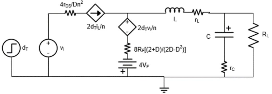
Figure 2.5: The averaged, large-signal and small-signal model of full-bridge DC/DC converter.
