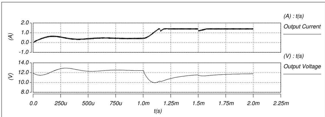
Figure 5.9: Simulated closed-loop output impedance step response.
