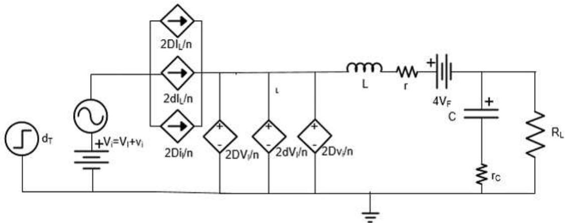
Figure 2.7: Model with explicit large-signal and small-signal switching components.
