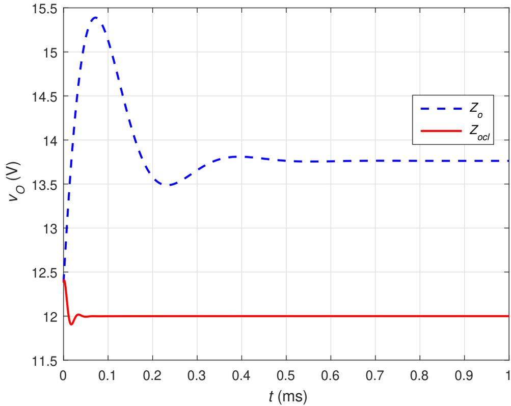
Figure 5.8: Calculated closed-loop output impedance step response, versus open-loop output impedance step response.
