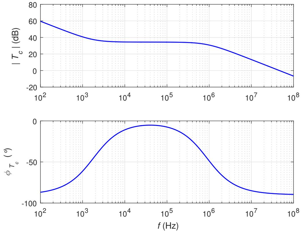
Figure 4.11: Calculated frequency response for the Type II controller transfer function.
