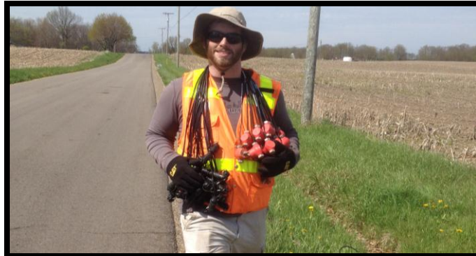
Figure 5: 4.5 Hz single-component geophone was deployed to receive the seismic signal for the study.
