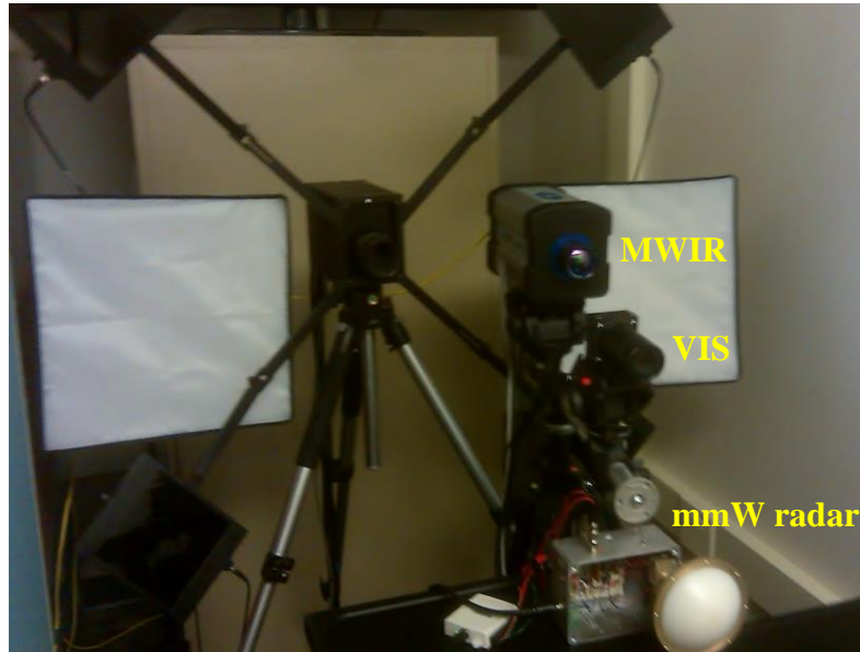
Figure 3.6. Subject's view of the imaging system. The MWIR camera is positioned six feet from the subject and aligned with the VIS camera such that the face and neck fill the field of view of each imager. The mmW radar system sits on a stand four feet from, and aligned with the subject's chest.
