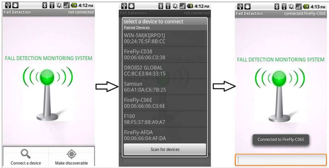
Figure 4.8: pairing the android app with the fall detection device
