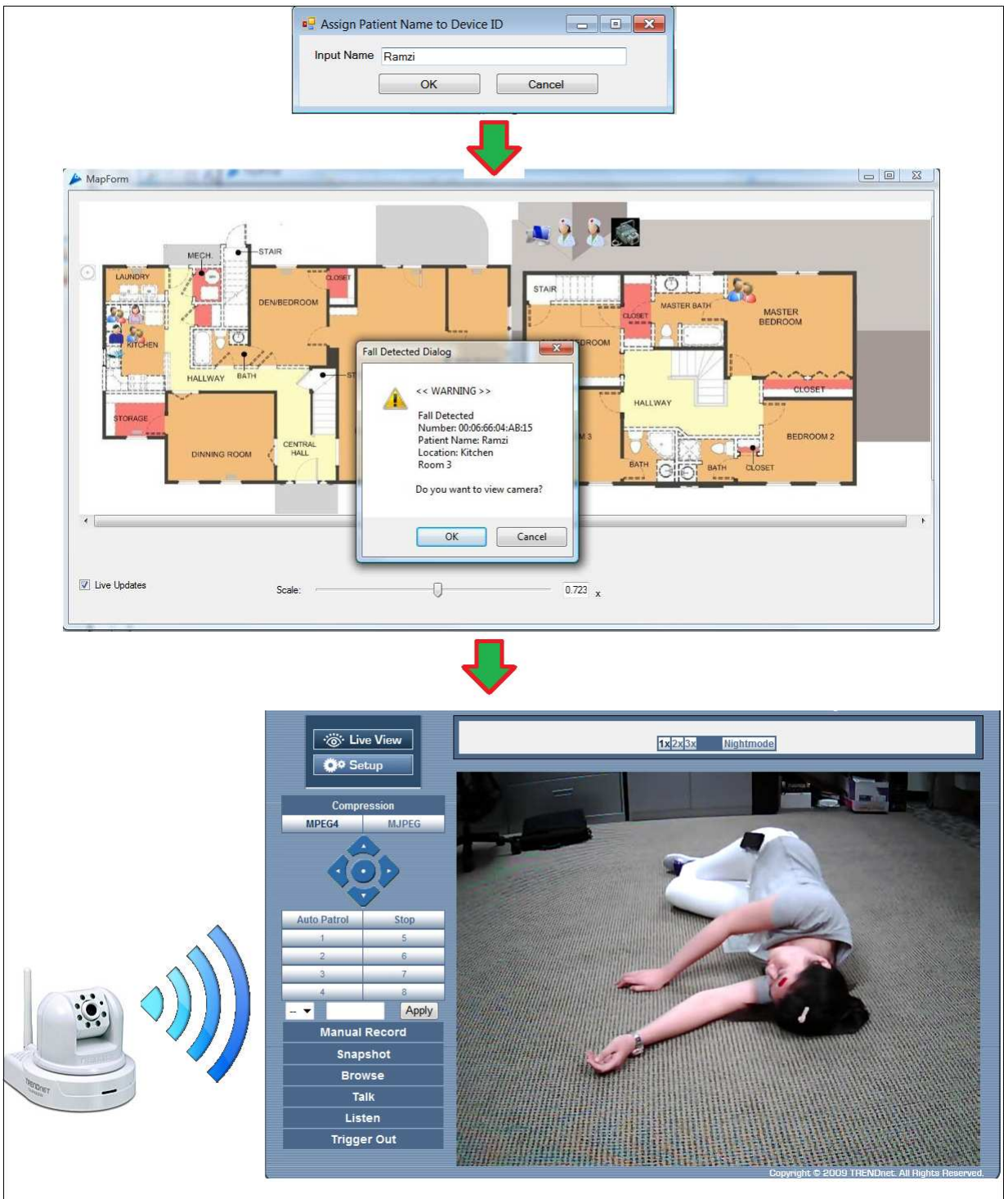
Figure 4.13: FastFind fall detection application with camera view
