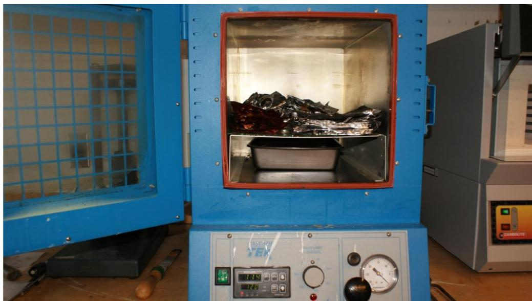
Figure 3.7 Vacuum Oven (Cascade Tek)
