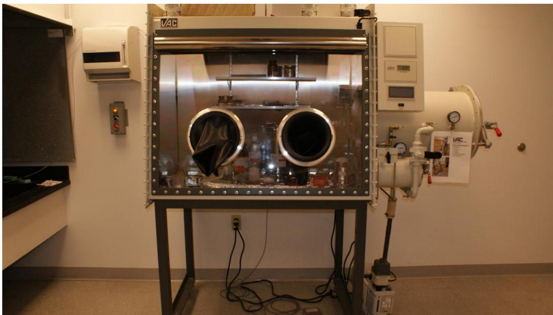
Figure 3.2 Glove Box (Vacuum Atmospheres Company).
