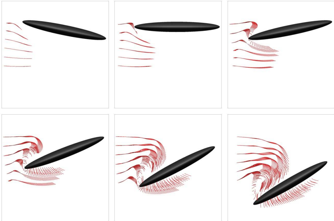
Figure 3.12: Six streak line seed curves begin to capture the leading edge vortex with many unnecessary particles.
