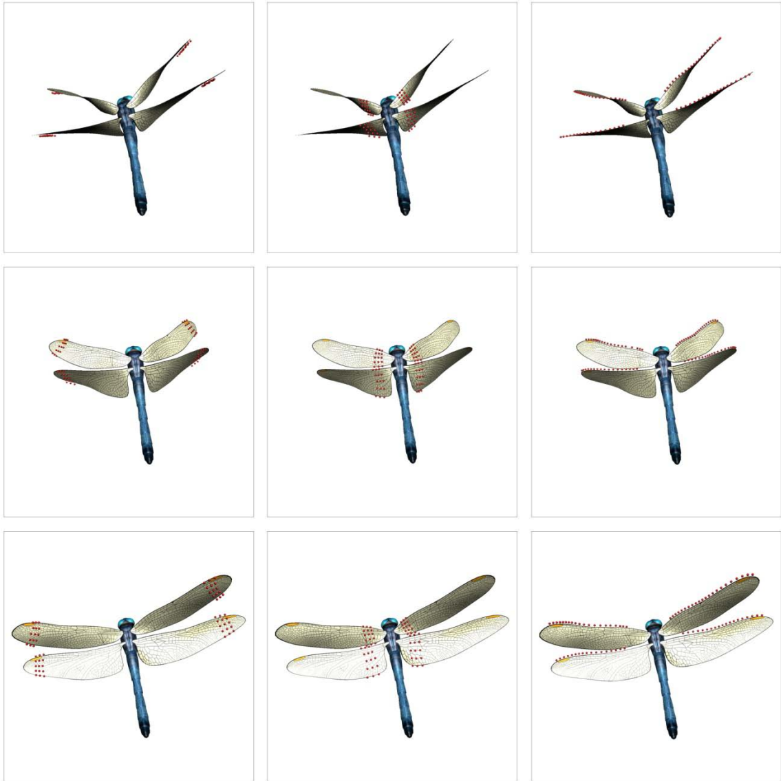
Figure 3.22: Vertex normal seeds placed at the wing tips (first column), wing root (second column) and leading edge (third column) shown at three different time steps.
