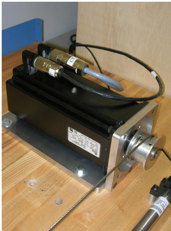
Figure C8: DC Servo Motor
