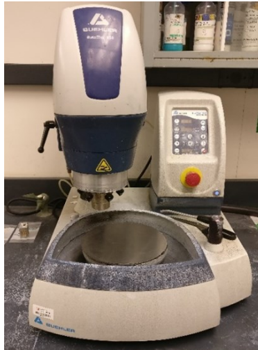
Figure 3.3: Buehler Ecomet 250 system used for polishing the distinct 304L SS specimens studied in this dissertation research work.
