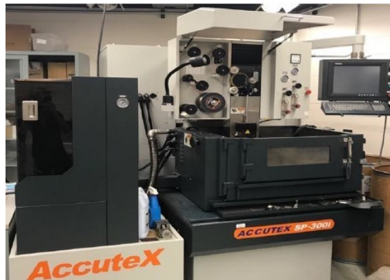
Figure 3.4: Accutex SP-300I electric discharge machine used for sectioning the various 304L SS specimens.
