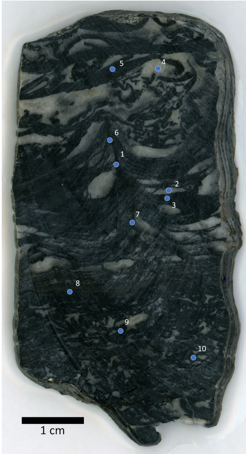
Figure III-2. Unpolished slab of sample KUR, oriented with the stratigraphic up position at the top. Blue dots indicate Raman analysis spots. Their numbers correspond to the numbers in Figure III-4A and Table III-1.
