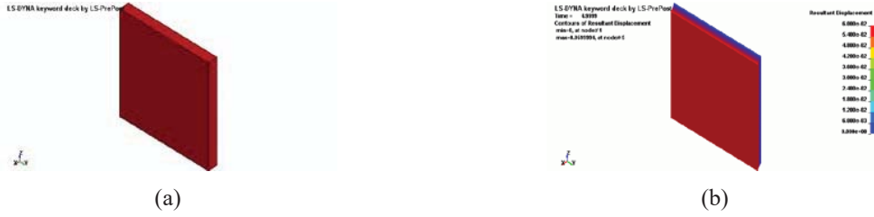
Figure 2.14 (a) finite element model of single cohesive element, (b) deformation on the front surface
