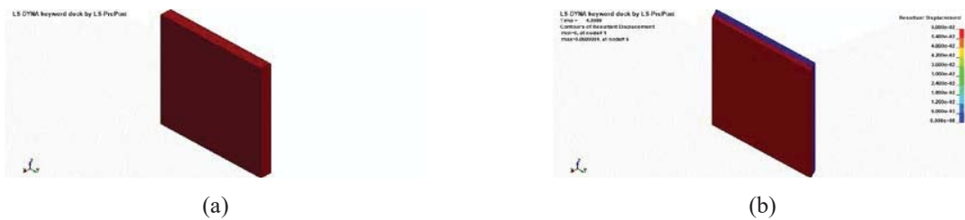
Figure 3.5 (a) finite element model, (b) prescribed motion on front side
