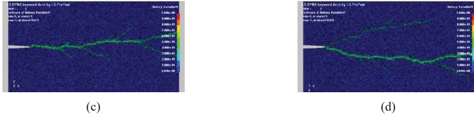
Figure 3.24 Damage factor results [0,1] considering strain rate, (a) 0.08 mm case, (b) 0.10 mm case, (c) 0.12 mm case, (d) 0.14 mm case
