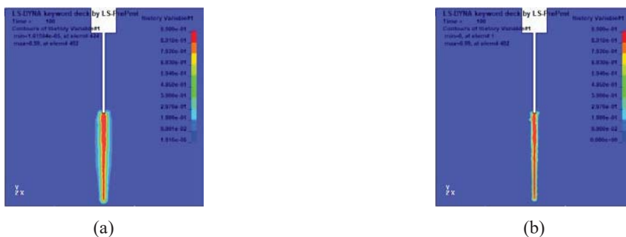
Figure 4.21 Phase result of the wedge splitting test, (a) classical phase field model, (b) length scale insensitive phase field model
