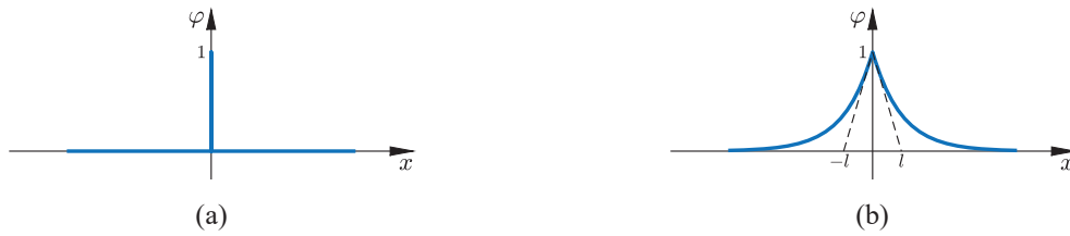
Figure 4.1 (a) non-smooth phase field, (b) diffusive phase field with length scale l
