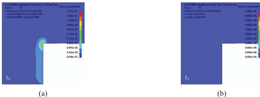
Figure 4.25 Phase result of the L-shaped panel test before fracture develops, (a) classical phase field model, (b) length scale insensitive phase field model
