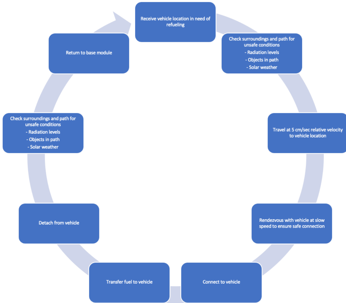
Figure 14 Mission Cycle Diagram for Refueling Vehicle
