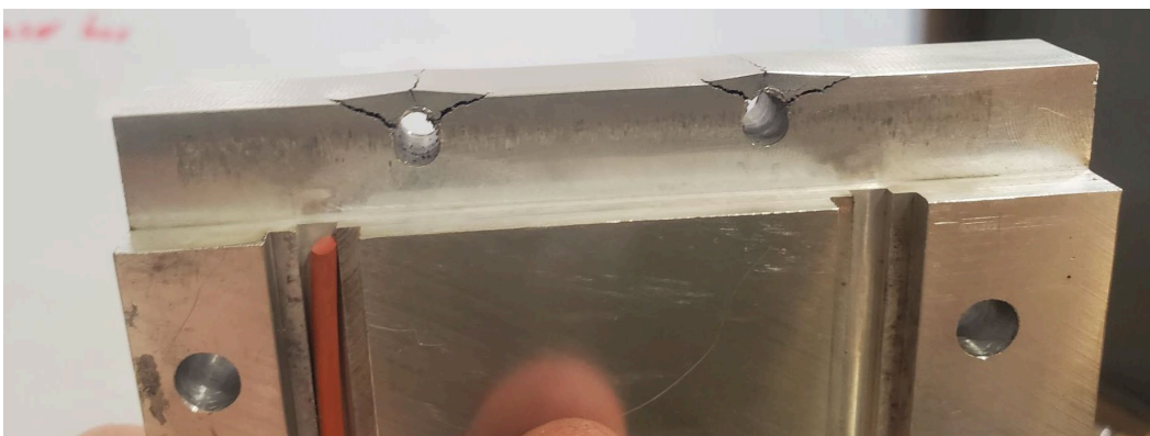
Figure 29: Damage to Redesigned Aluminum Top and Bottom Piece caused by end piece separation
