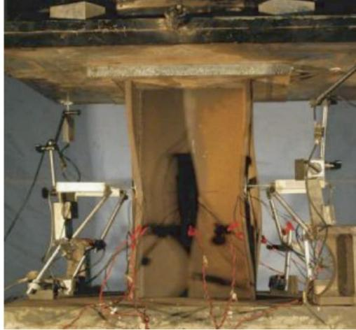
*Fig. 2: Local Buckling mode observed in one of the test specimens. (Shi et al., 2015)*
