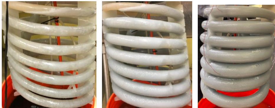
Figure 14. Frozen PCM Radius vs. Time for Latent (PCM) Experiment and Representative PCM Solidification Photos at Time = 1:20, 2:20, and 4:20 hours
