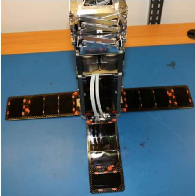
Fig. 3-6—Clyde Space’s 2U single-sided and double-sided deployable solar panels installed on CryoCube chassis.
