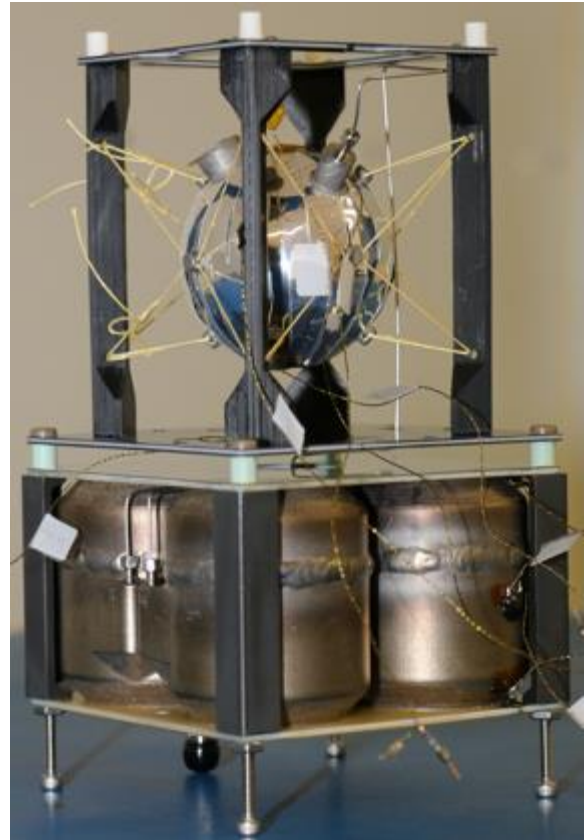
Fig. 1-3—CryoCube-1's gas pressure system is designed to liquefy gaseous Xenon at cryogenic temperatures.
