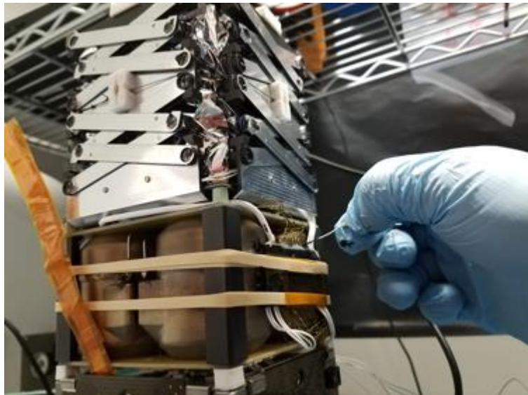
Fig. 7-6—Once the two halves of the spacecraft were mechanically mated together, final electrical connections were made between the experiment and electronics bus. Epoxy was used to rigidly attach the electrical connectors to the spacecraft.
