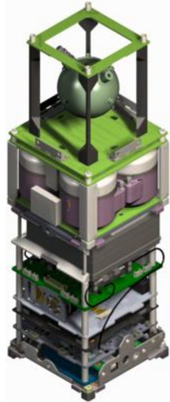
Fig. 7-1—A detailed solid model of the CryoCube-1 system was used to help design and package all subsystems within the CubeSat.
