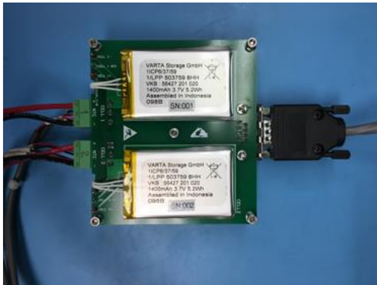
Fig. 7-7—Flight battery cells were charged and discharged using a custom-made test setup.
