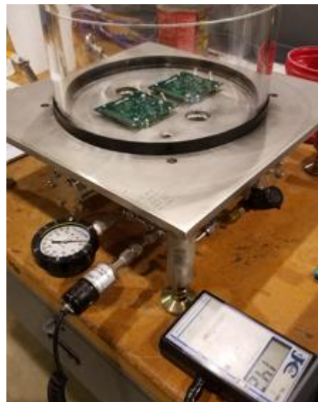
Fig. 7-9—Flight battery cells were exposed to vacuum conditions under a small bell jar.
