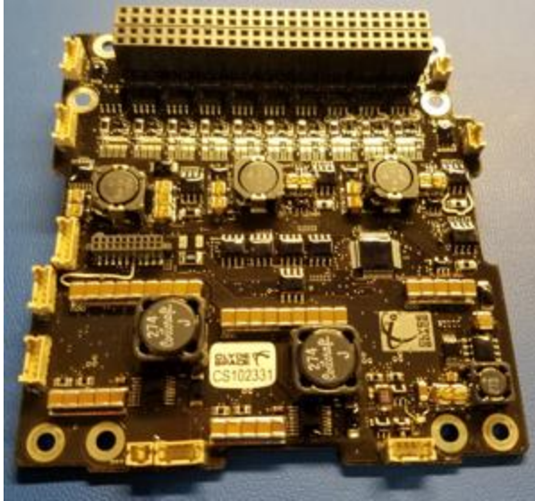
Fig. 3-8—The Clyde Space 3 rd Generation EPS is used to charge batteries and distribute electrical power to CryoCube-1's electrical subsystems.
