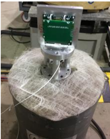
Fig. 7-8—Flight battery cells were exposed to vibration in all three axes.
