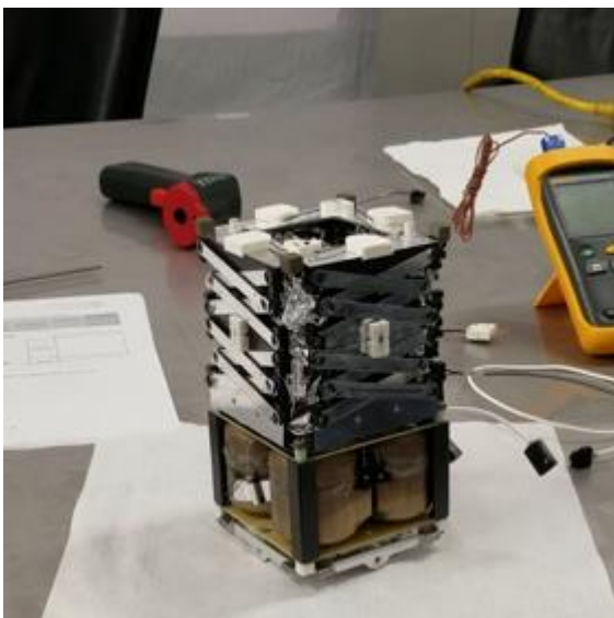
Fig. 7-11—Prior to deployment, the sunshield fits within a 1U volume.
