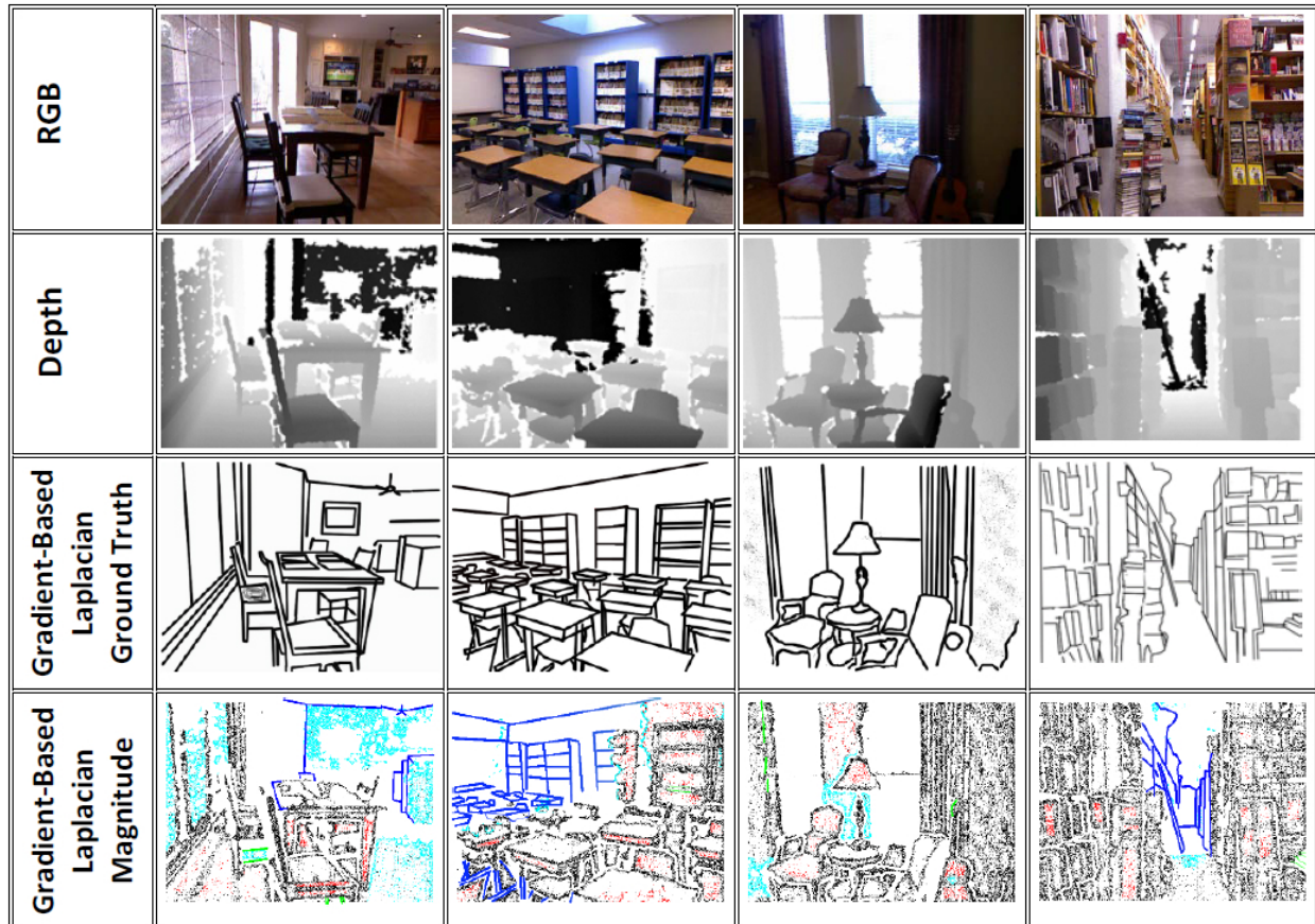
Figure 4.4: This figure shows the edge detection results of the Gradient Based Laplacian magnitude operators on the NYU Depth data set. Black, red, green, light blue, and dark blue pixels represent the true positives, false positives caused by algorithm, false negatives caused by algorithm, false positive caused by noise, and false negative caused by noise, respectively.
