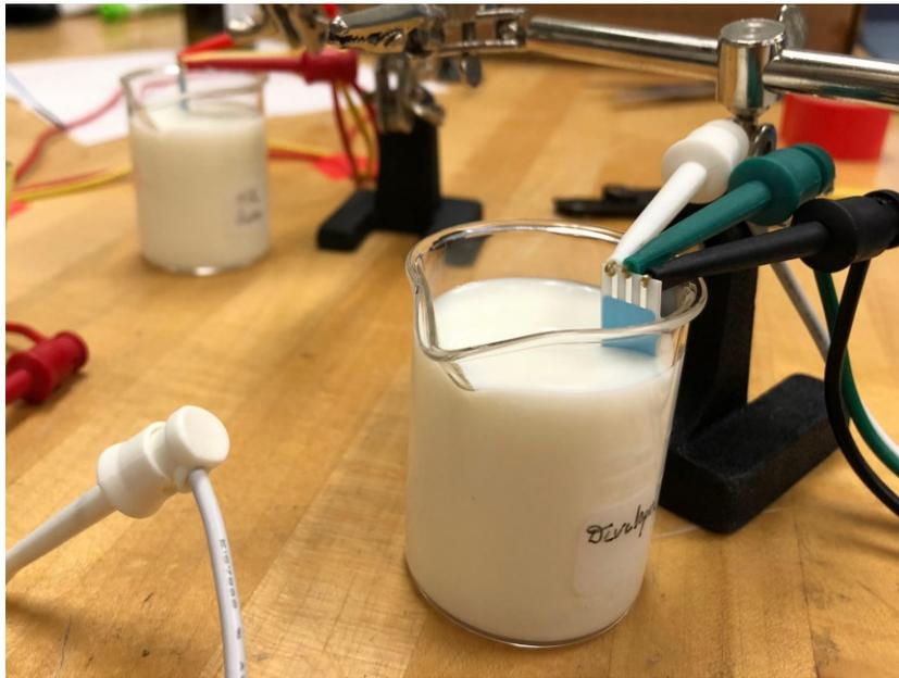
*Figure 5-12 Experimental set up for simultaneous testing of two screen printed electrochemical cells*
