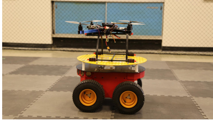
Figure 4.1: The test sUAV with the mobile target platform.
