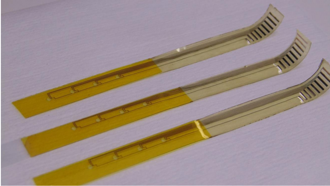
Figure 5-4. Fabricated pressure sensor array.
