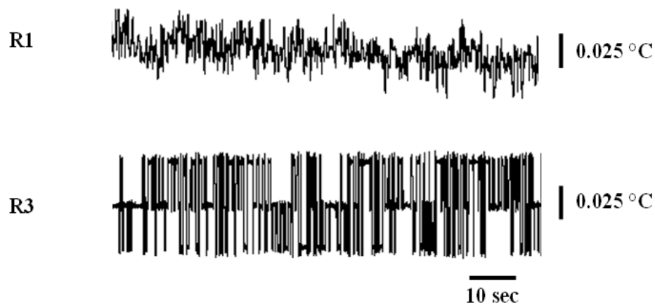
Figure 3-13. Measured in vivo noise level for polysilicon thermistors: R_1 with the dimension of 20\text{ }\mu\text{m} \times 160\text{ }\mu\text{m} : 0.025\pm 0.03\text{ }^\circ\text{C} ; R_3 with the dimension of 200\text{ }\mu\text{m} \times 160\text{ }\mu\text{m} : 0.07\pm 0.06\text{ }^\circ\text{C} .
