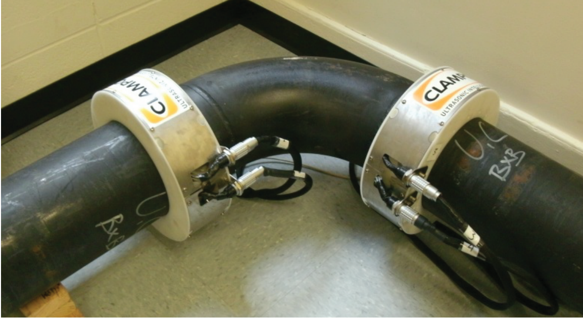
Figure 6-1: Example of inspection configuration for guided wave tomography of pipe bends. Two ring arrays of ultrasonic transducers are mounted at the ends of the bend along the straight sections of the pipeline. Transmit-receive pairs are then formed with the transducers of the two arrays to propagate guided wave signals inside the thickness of the pipe wall and across the bend.
