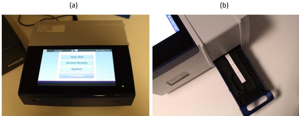
Figure 5-1 External LFIA reader: (a) Qiagen reader with a LCD display; (b) Reader with slot to insert an LFIA strip.
