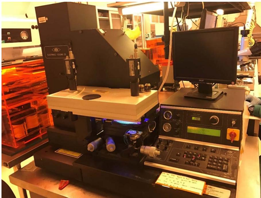
*Figure 2-8 UV exposure tool used for Photolithography*
