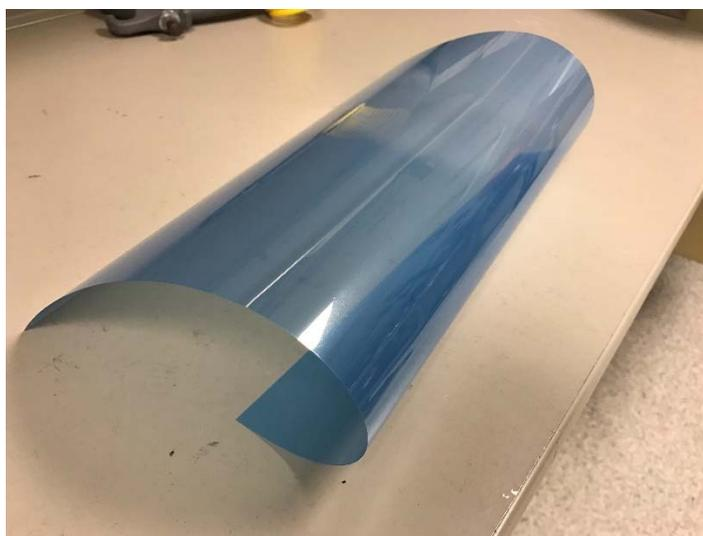
*Figure 2-7 ITO coated sheet obtained from Sigma Aldrich (blue color due to liner).*
