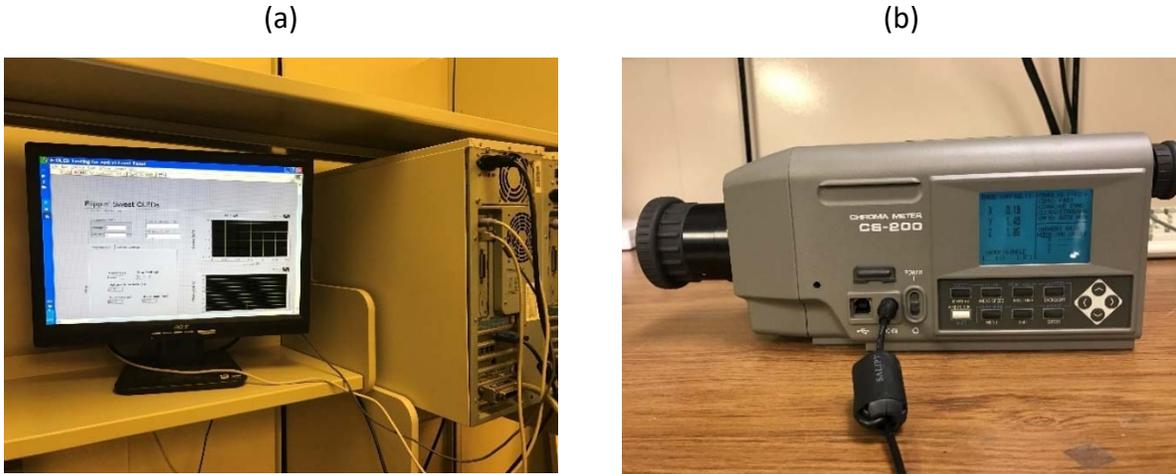
Figure 2-12 OLED characterization setup; (a) LabVIEW PC control; (b) Brightness measurement meter (minolta)
