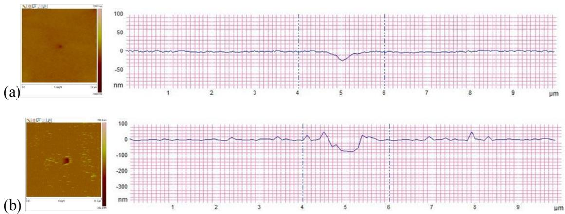
**Figure 5.15: Nanocutting machining results on a) Silicon and b) Borosilicate Glass**
