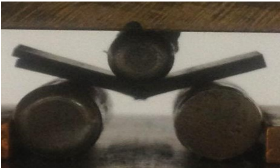
Figure 3.13. Short beam shear (SBS) test showing shear failure mode at the mid plan where the maximum shear stress occurs.
