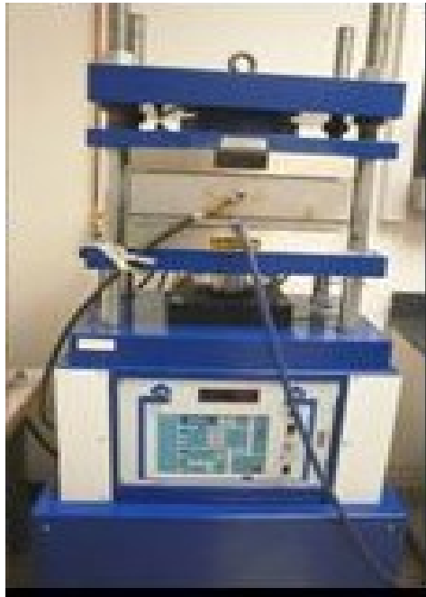
Figure 3.6. Automated composite press machine for composite fabrication process.
