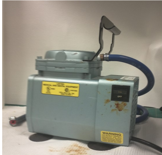
Figure 4.3. Image of vacuum pump used for composite laminate consolidation.
