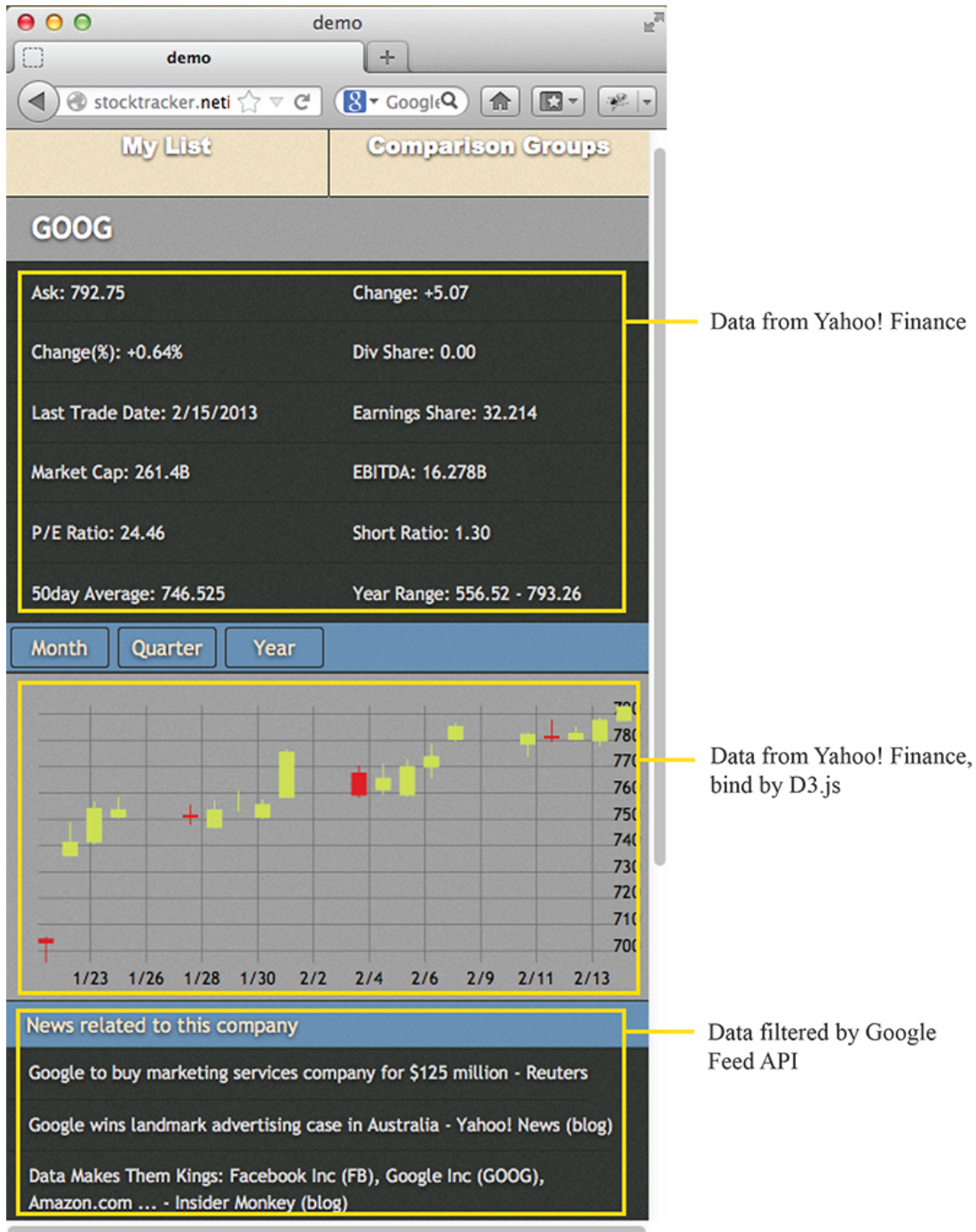
Figure 20. The connection between application interface and database
