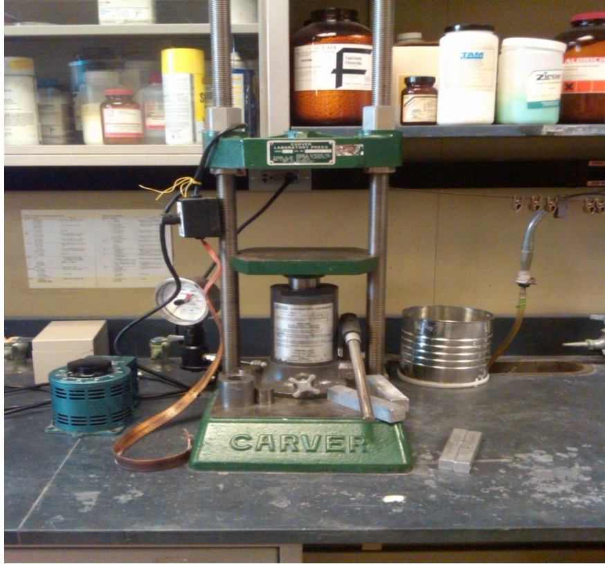
Figure 15: Carver Laboratory equipment Model 3192 Die Press
