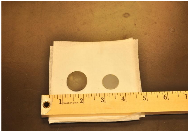
Figure 16: Composite pellets pressed on the die press
