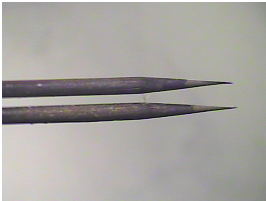
Figure 71: Tungsten electrodes insulated with aluminum oxide and mounted in acrylic glass block, showing final electrode separation
