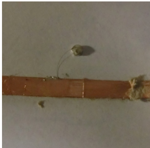
Figure 7: Mounting of copper contact strips to end of CNT thread
