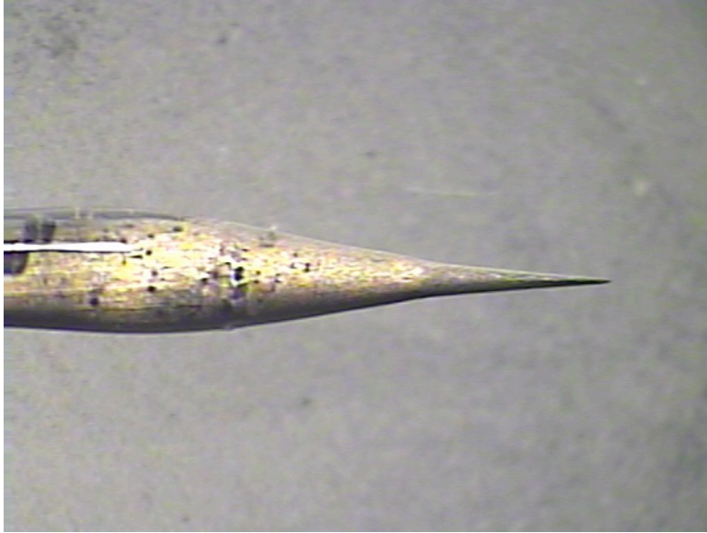
Figure 75: 1 of 2 epoxy insulated tungsten electrodes (epoxy is shiny region)
