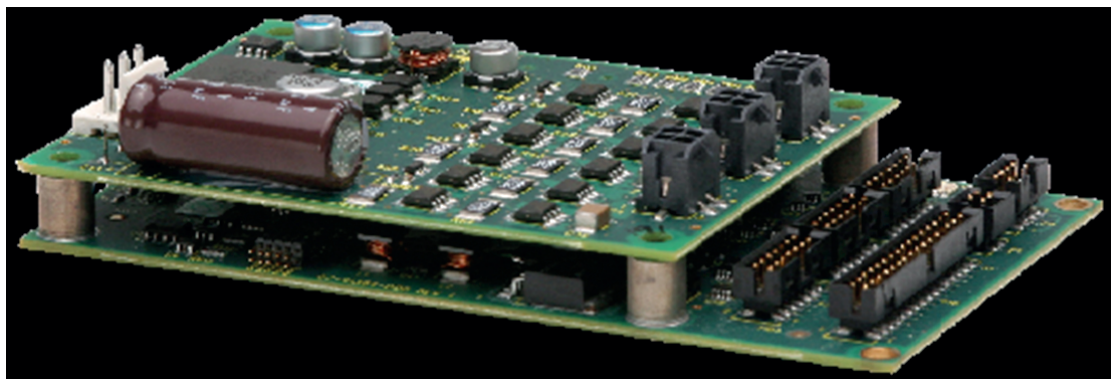
Figure 26 - Stepnet ST3 controller [60]
