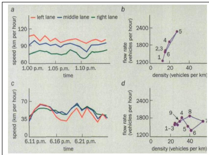
**Figure 10: Comparison between free flow (a, b) and synchronized flow (c, d)**
