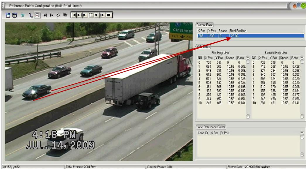
**Figure 21: Demonstration of vehicle length data extraction using VEVID**
