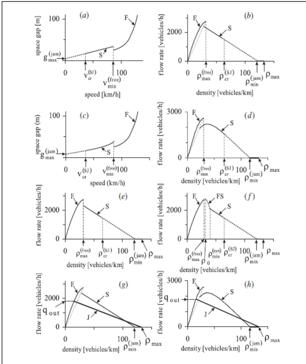
**Figure 9: Steady state Speed Adaptation (SA) model**
