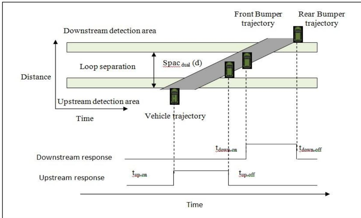
**Figure 7: Time-space representation of loop detector pulses**
