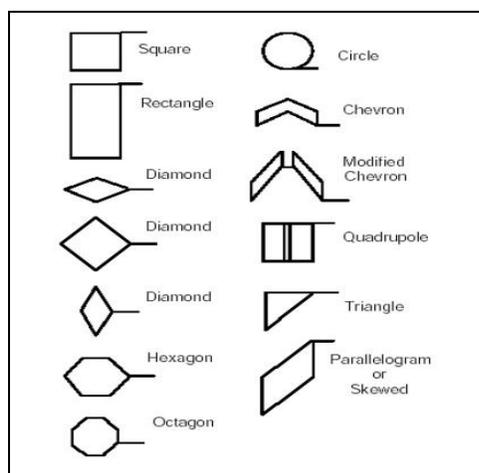
**Figure 4: Different loop detector shapes**
