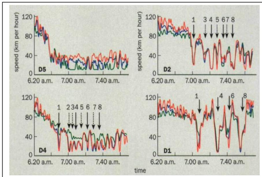
**Figure 11: Speed pattern observed during stop-and-go flow**
