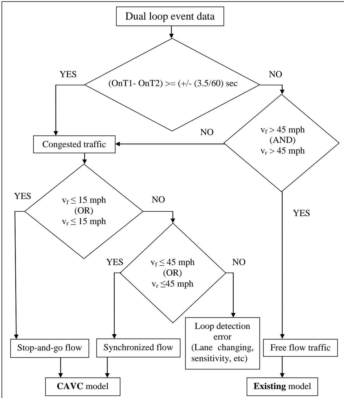
**Figure 25: Traffic flow state identification methodology used in CAVC model**
