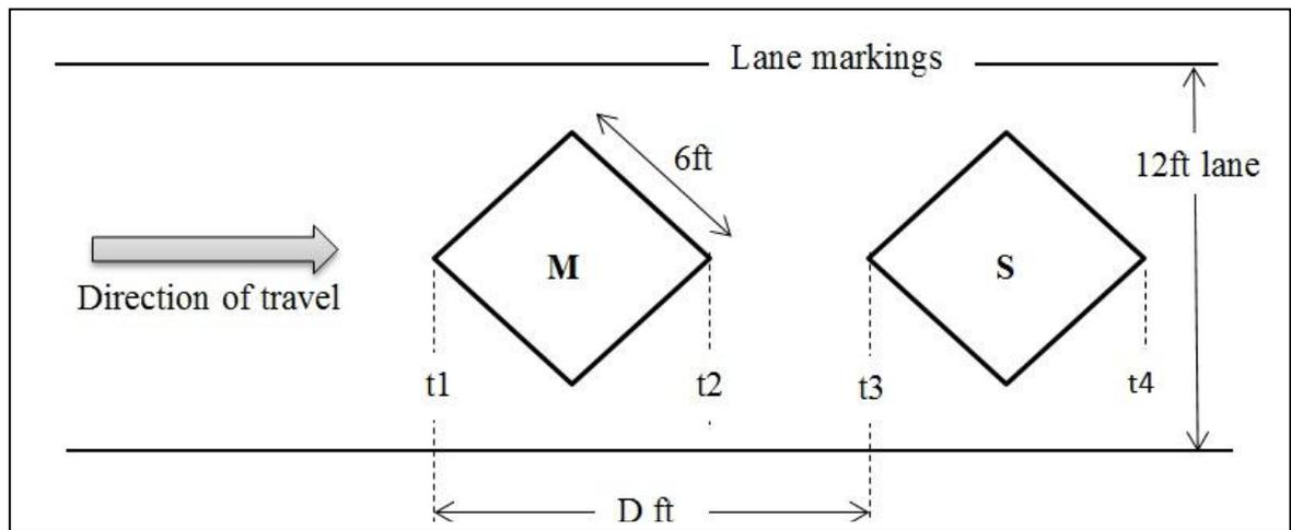
**Figure 6: Layout of typical dual loop detector**
