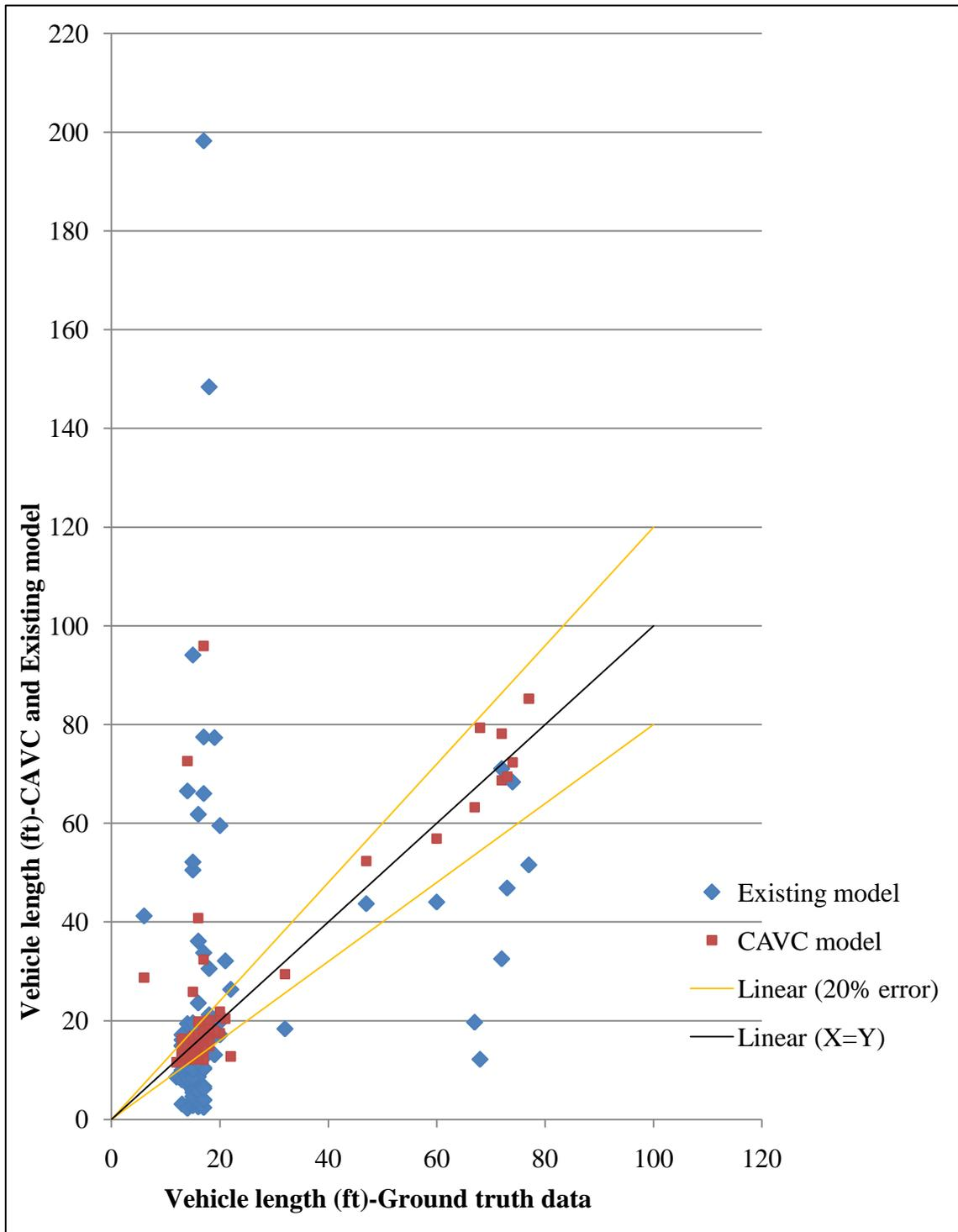
**Figure 27: CAVC and Existing model vs Ground truth data (stop-and-go flow)**
