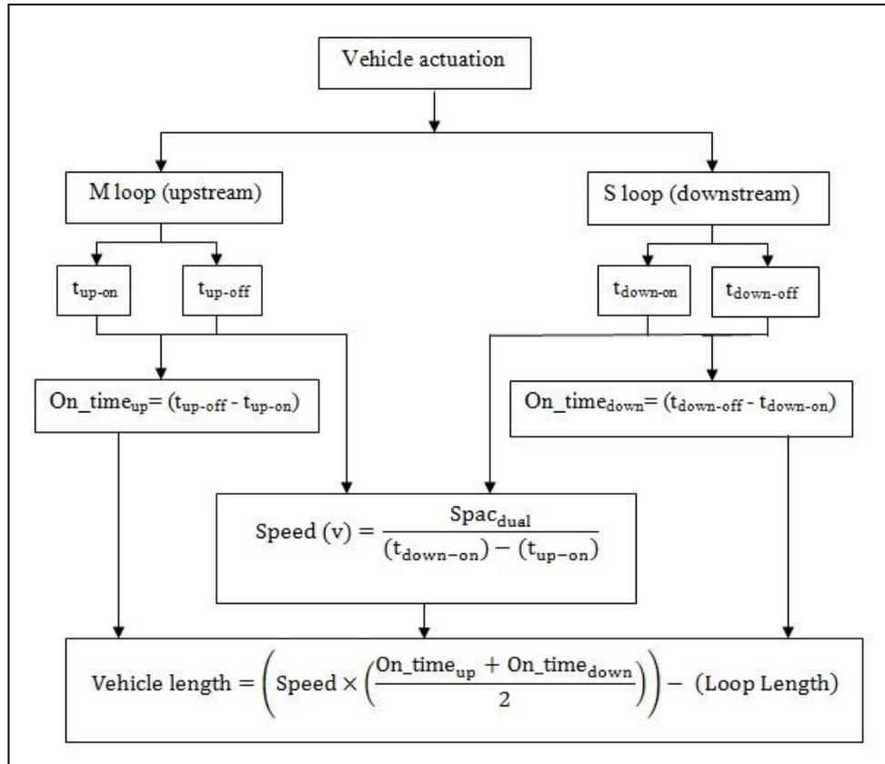
**Figure 8: Existing length based vehicle classification model**
