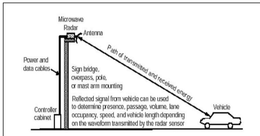
**Figure 2: Microwave radar operation**
