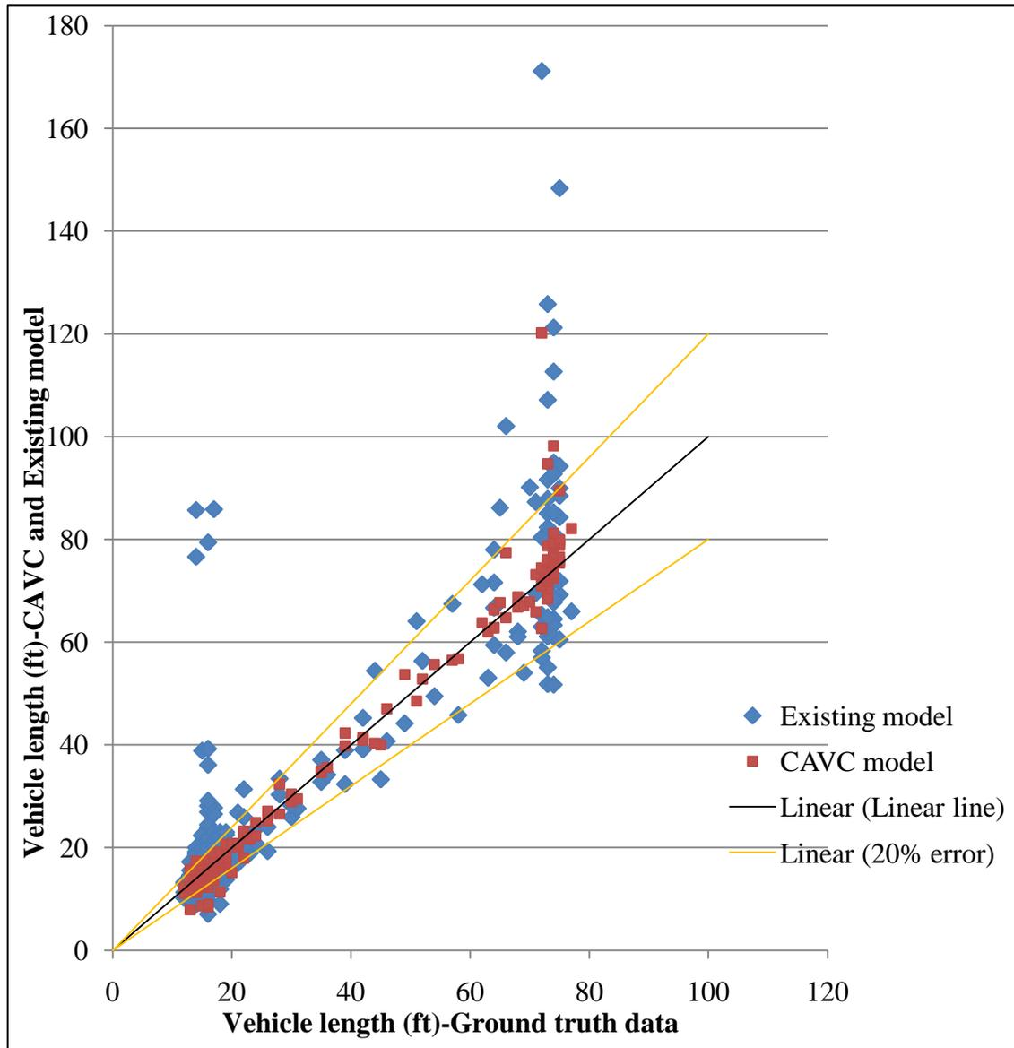
**Figure 26: CAVC and Existing model vs Ground truth data (synchronized flow)**
