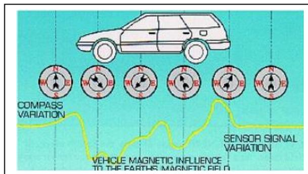
**Figure 5: Perturbation of Earth's magnetic field by ferrous metal vehicle**
