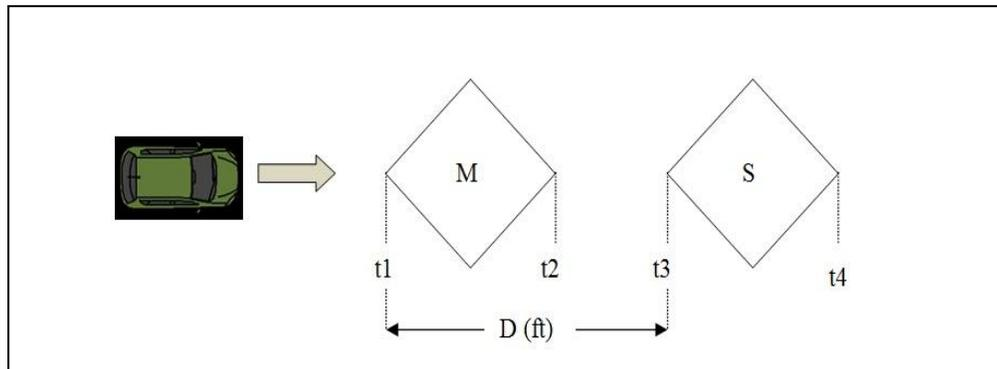
**Figure 24: Layout of dual loop detectors**
