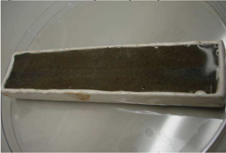
Figure 5. Cement-lined coupon with spore suspension
