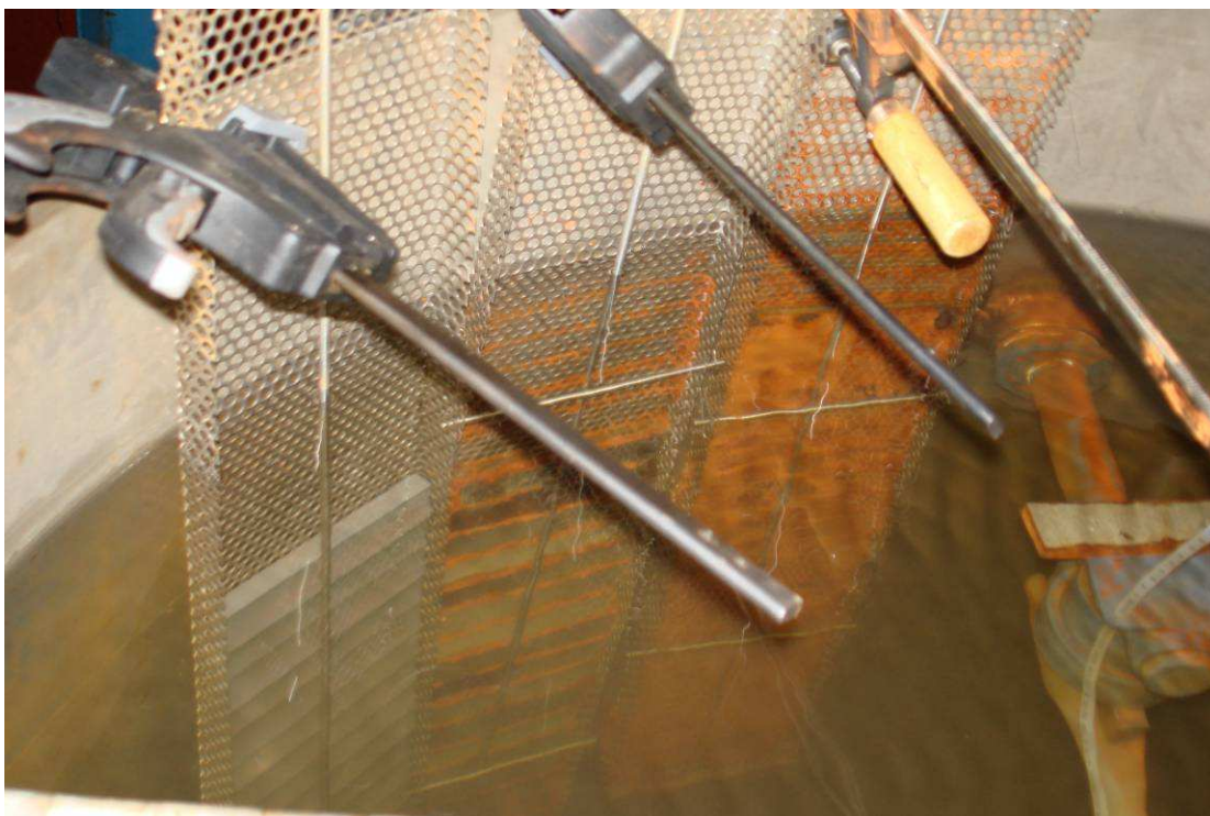
Figure 1. Racks holding coupons in recirculation tank. Pipe material (from left to right) is PVC, cement-lined, and iron.
