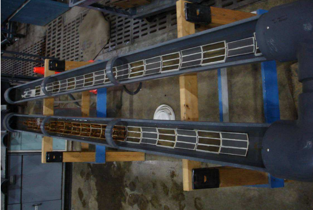
Figure 6. Coupons conditioning in Cincinnati tap water (note that covers have been removed for photo and iron coupons were kept downstream from other coupon materials so the corrosion would not contaminate them)
