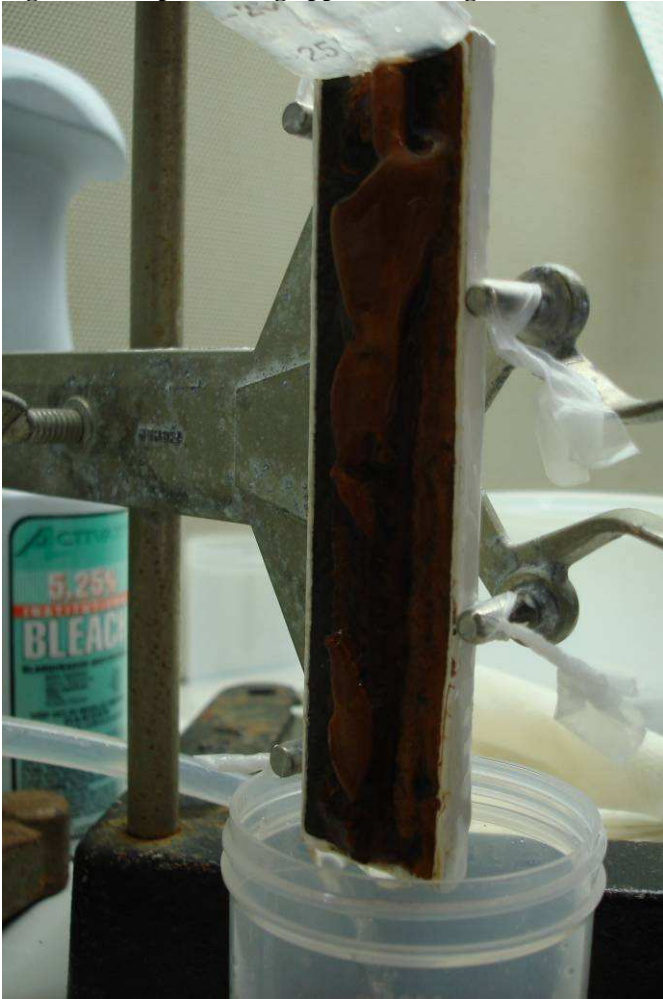
Figure 7. Coupon rinsing apparatus using buret stand
