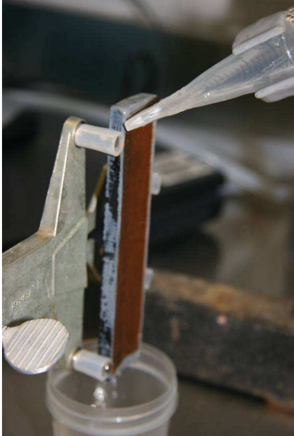
Figure 13. Collecting rinse tap water with buret stand and modified 30 mL syringe
