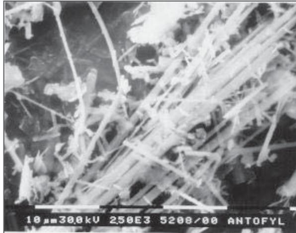
Figure 7: Cluster of asbestos fibers
