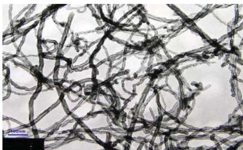
*A TEM image of our Multi Walled Nanotubes-MWNTs 95wt% 20-30nm OD*
