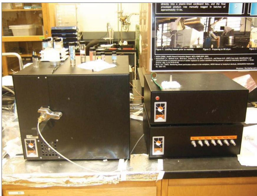
Figure 19: Sunset Laboratory OC-EC Thermal-Optical Analyzer
