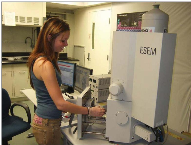
Figure 34: Scanning Electron Microscope (FEI/Phillips XL30 ESEM-FEG) at the University of Cincinnati
