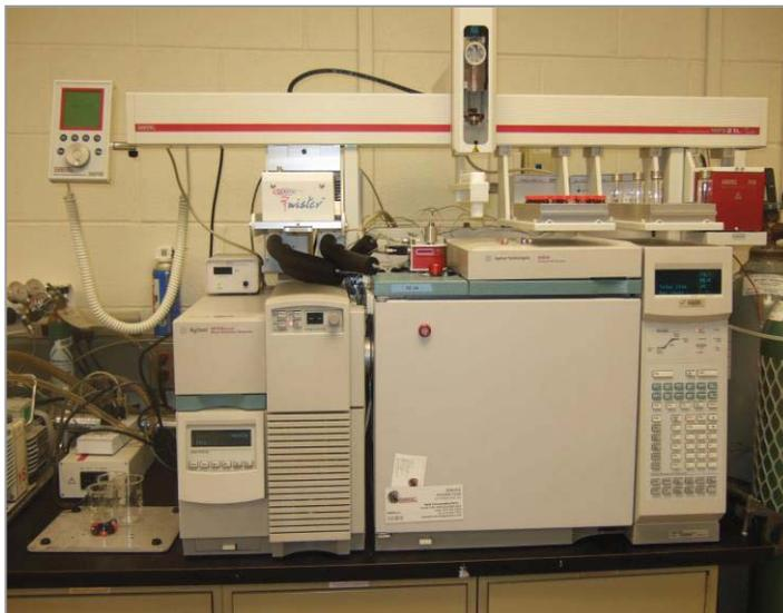
Figure 50: GC/MS located at NIOSH Cincinnati
