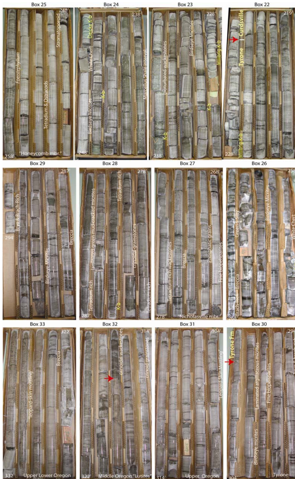
Figure 11: Photographs of KGS-C204, Lawrenceburg, Kentucky (Anderson County) core showing the Oregon through Curdsville interval. Portions of the upper lower Oregon, middle Oregon, Upper Oregon, and the entire Tyrone are displayed. Key K-bentonite horizons and other marker units are identified in the Tyrone as discussed in the text.
