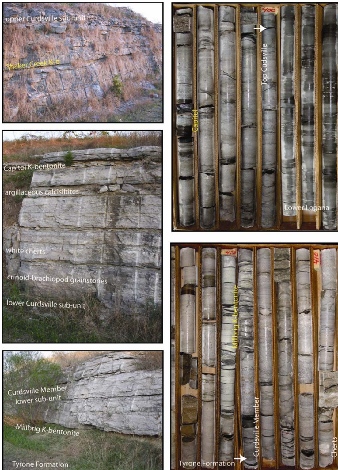
Figure 14: Outcrop exposures and core photographs for the Curdsville Limestone. Outcrop photographs are taken from the KY-HWY 68 road cut at Shaker Creek, Kentucky and the reference section for the Shaker Creek K-bentonite. Core photographs are of the Ohio DCNR Core 3020 in Hamilton County, Ohio. The pattern and development of the Curdsville between these localities (some 100 km apart) shows remarkable similarities and relatively uniform thickness between these areas.
