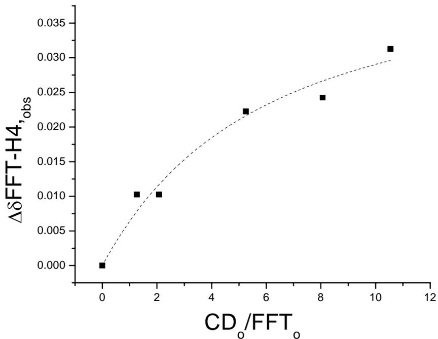
**Figure 2.6.** ■ Experimental binding isotherm generated from data of Table 2.2 --- Best fit curve of nonlinear regression analysis according to Equation (2.6).
