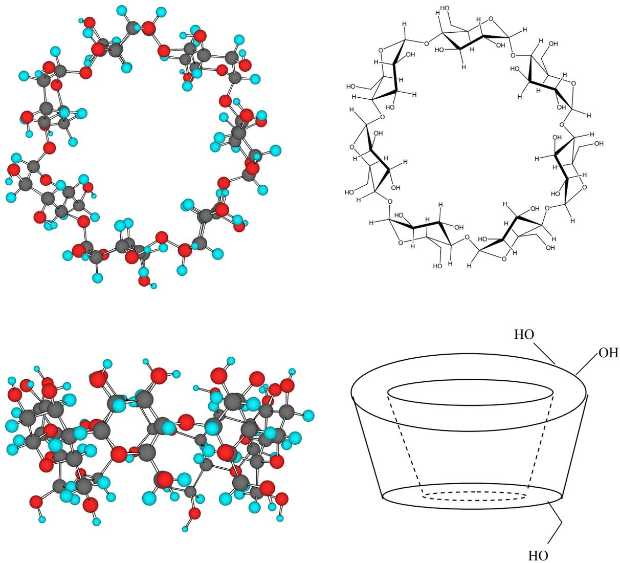
**Figure 1.2.** Schematic representation of the individual molecular dimension of  $\alpha$ -,  $\beta$ -, and  $\gamma$ -CD.
