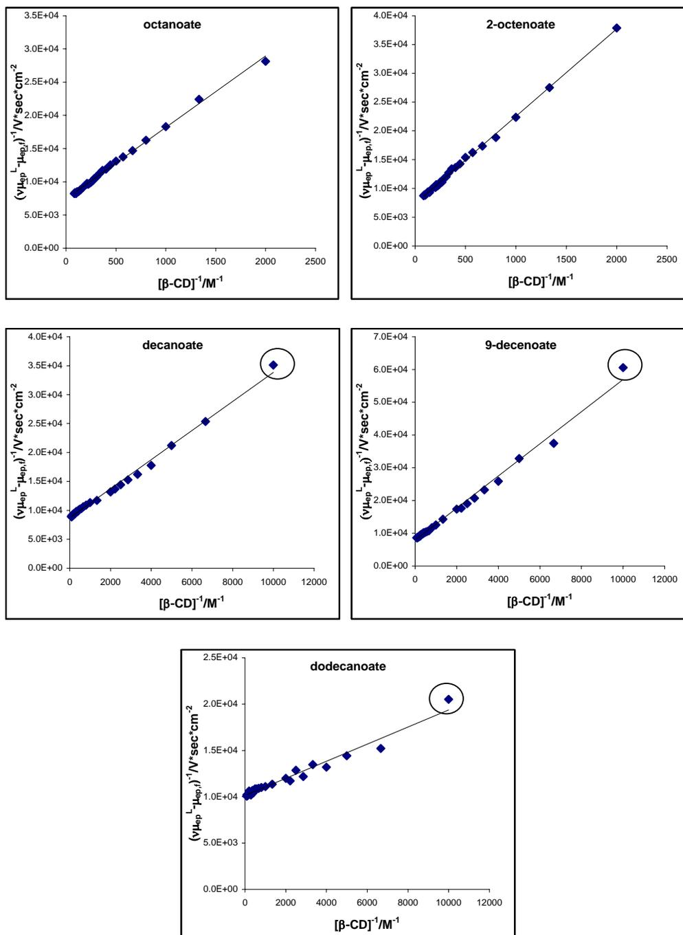
**Figure 3.5.** X-reciprocal plots used to investigate sample overloading (ligand saturation) at the lower  $\beta$ -CD concentrations employed in the BGE. Circled points are excluded from the dataset before binding parameters are calculated.
