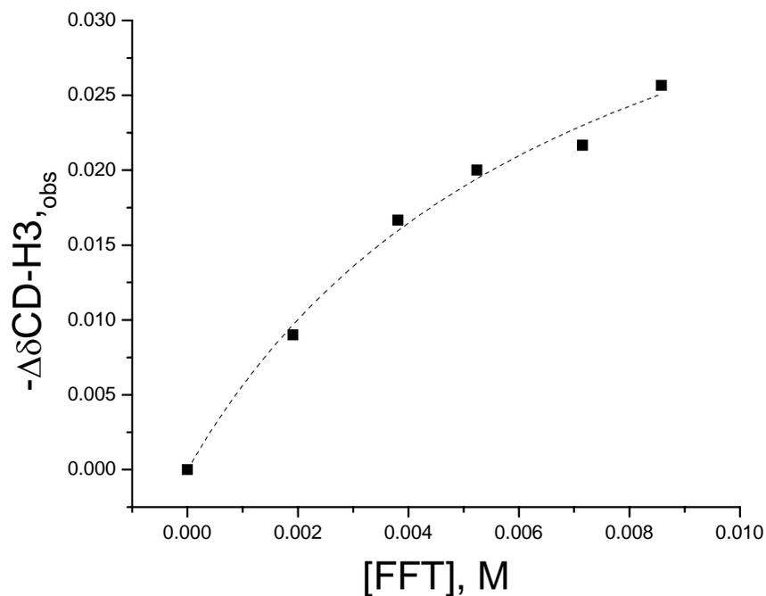
**Figure 2.5.** ■ Experimental binding isotherm generated from data of Table 2.2. --- Best fit curve of nonlinear regression analysis according to Equation (2.6).
