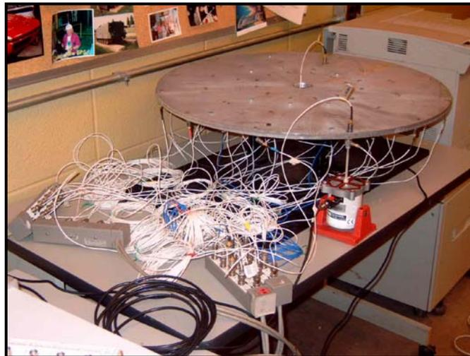
**Figure 5.7 - Experimental set up for the lightly damped circular plate**
