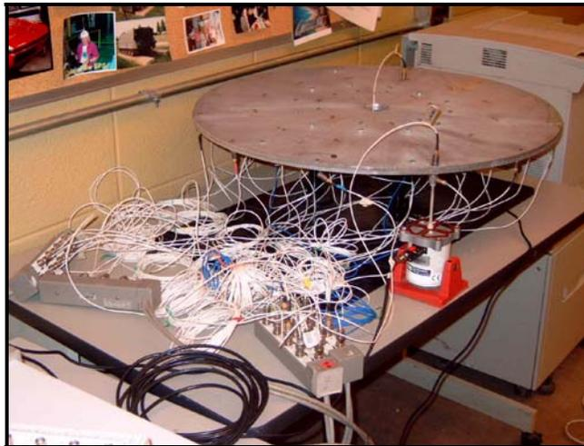
**Figure 3.3: Experimental set up for the lightly damped circular plate**
