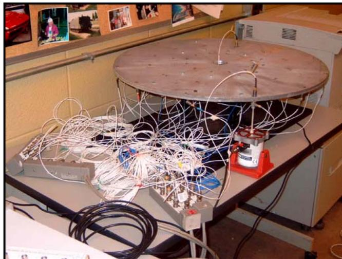
**Figure 4.10: Experimental set up for the lightly damped circular plate**
