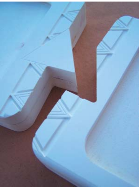
Figure 18. Final patterns milled into prototype.
