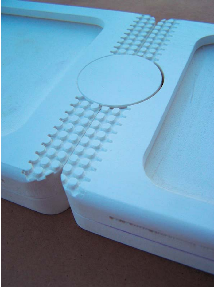
Figure 20. Final patterns milled into prototype.
