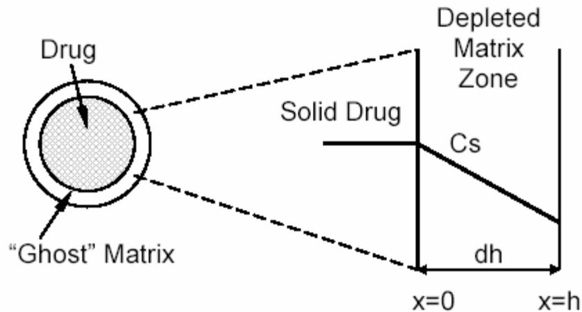
**Figure 1. Schematic representation of a matrix release system**
