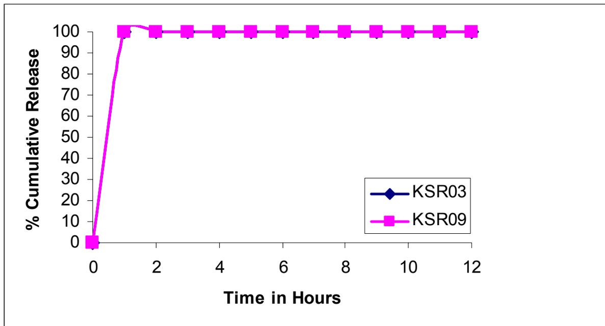
**Figure 20. Effect of high levels, >50%, of dicalcium phosphate excipient on dextromethorphan release from ER matrix tablets. (plotted values are average values, n=8, RSD<4%)**
