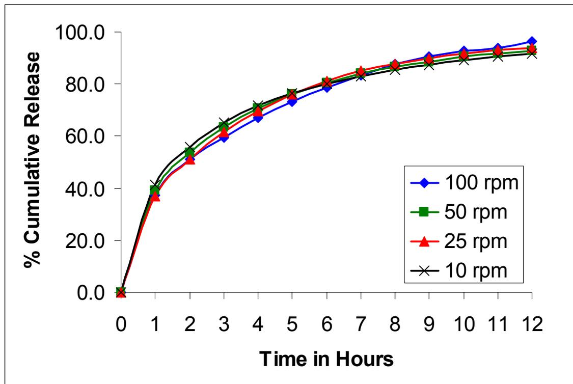
Figure 41. In vitro dissolution profiles of HPMC/Eudragit ER matrix tablets at variable dissolution agitation rates. (plotted values are average values, n=8, RSD<3%)
