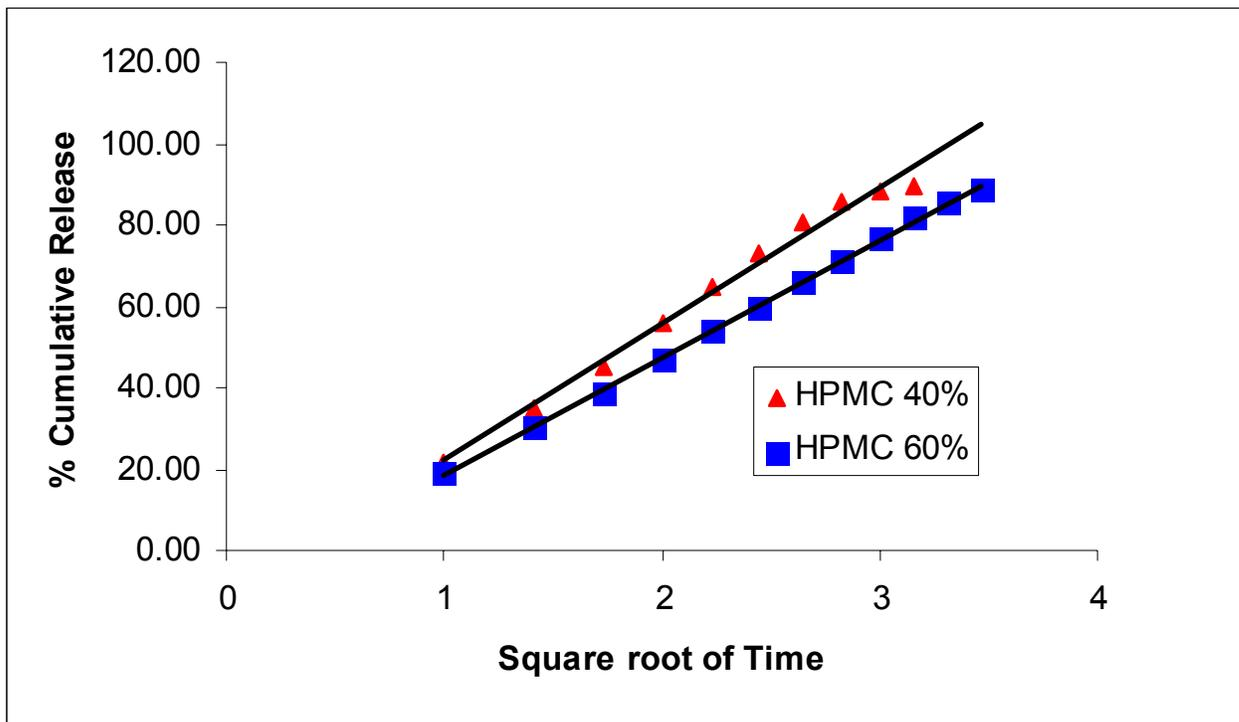
**Figure 11. Effect of HPMC on diffusion controlled dexamethorphan release from ER matrix tablets**
