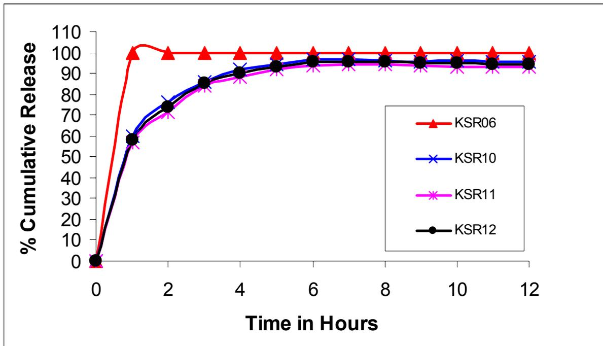
Figure 23. Effect of PVAP on dextromethorphan release from ER matrix tablets. (plotted values are average values, n=8, RSD<4%)
