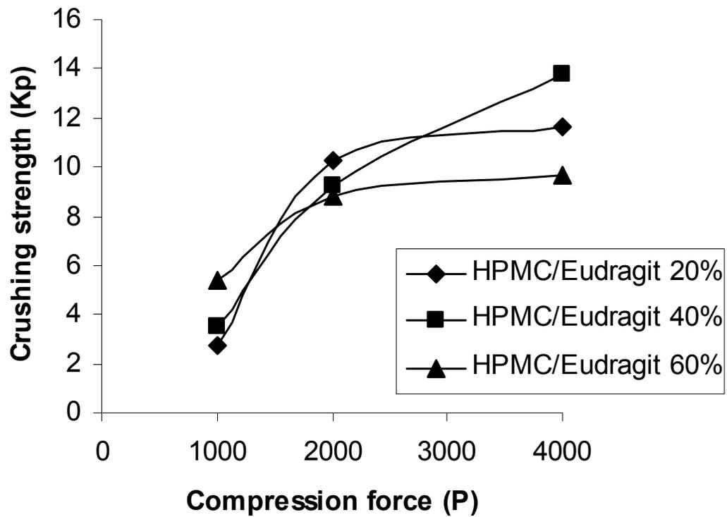
**Figure 9. Effect of compression force on the hardness (crushing strength) of HPMC/Eudragit tablets**
