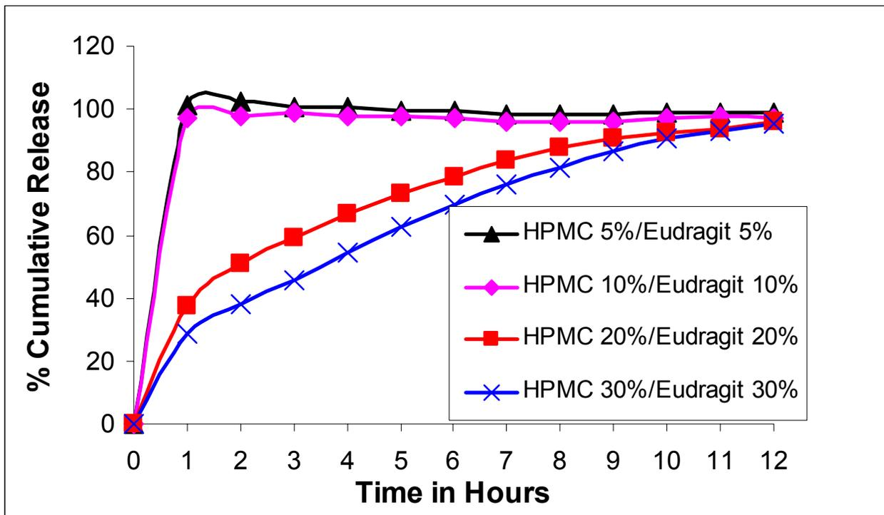
Figure 14. Effect of HPMC/Eudragit combination blends on dextromethorphan release from ER matrix tablets. (plotted values are average values, n=8, RSD<3%)
