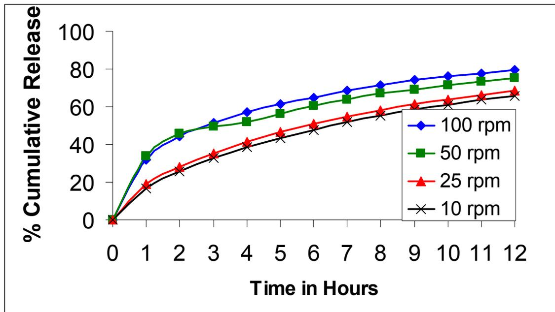
Figure 42. In vitro dissolution profiles of PVAP ER matrix tablets at variable dissolution agitation rates. (plotted values are average values, n=8, RSD<3%)
