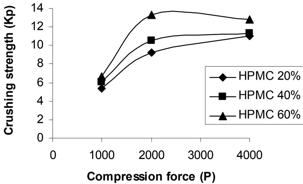
Figure 7. Effect of compression force on the hardness (crushing strength) of HPMC tablets
