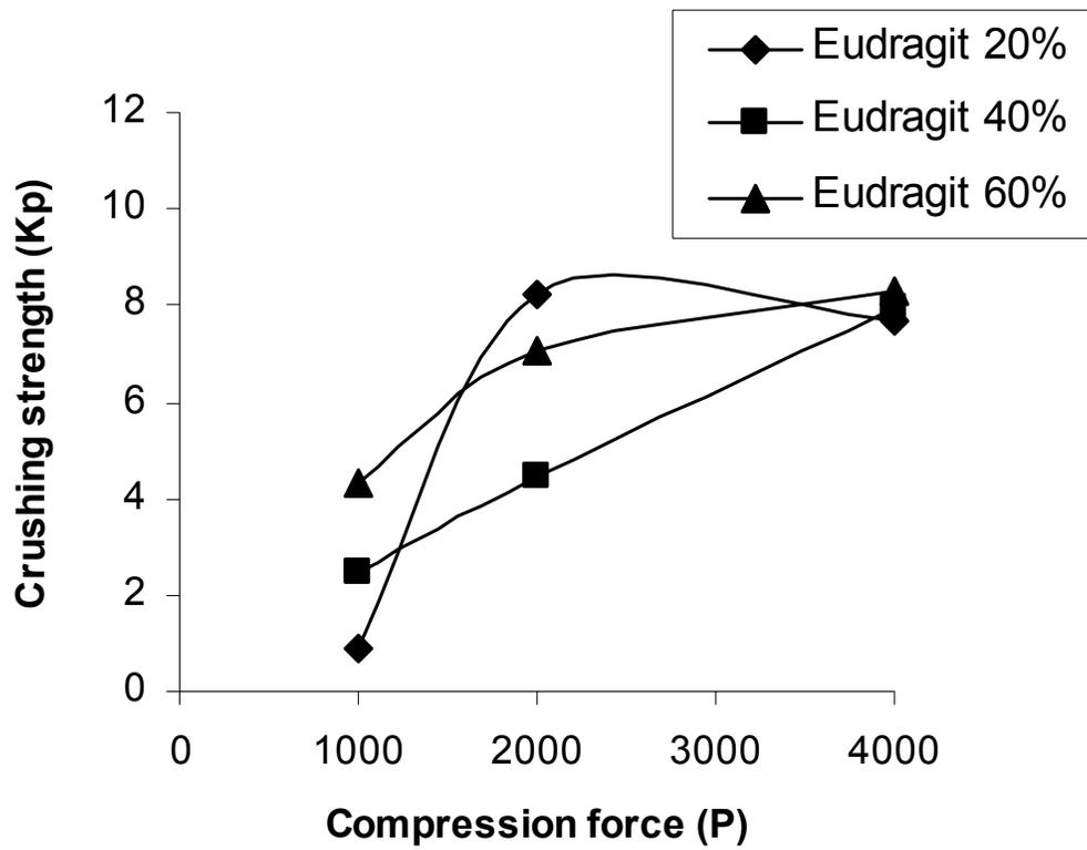
Figure 8. Effect of compression force on the hardness (crushing strength) of Eudragit tablets
