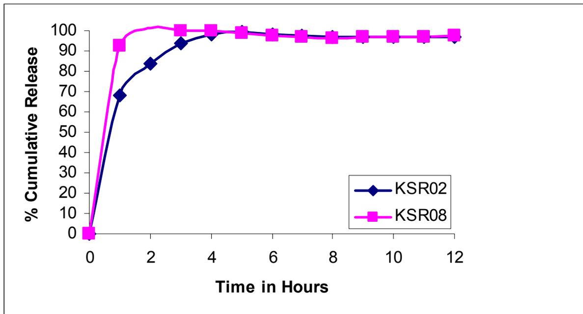
**Figure 19. Effect of high levels, >50%, of microcrystalline cellulose excipient on dextromethorphan release from ER matrix tablets. (plotted values are average values, n=8, RSD<4%)**
