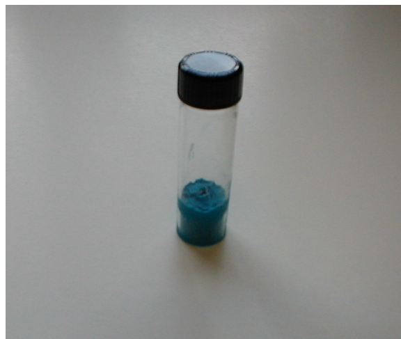
Fig. 8. Dye release vial with modeling clay/salt plug in place. Note hole in top of modeling clay.
