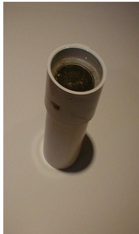
Fig. 4. Porous stone/adapter ring assembly installed in PVC
