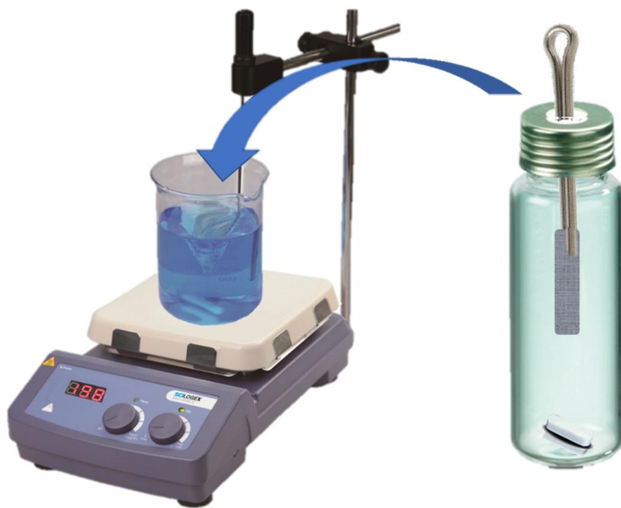
Figure 2-9 Diagram of the apparatus used for TF-SPME.
