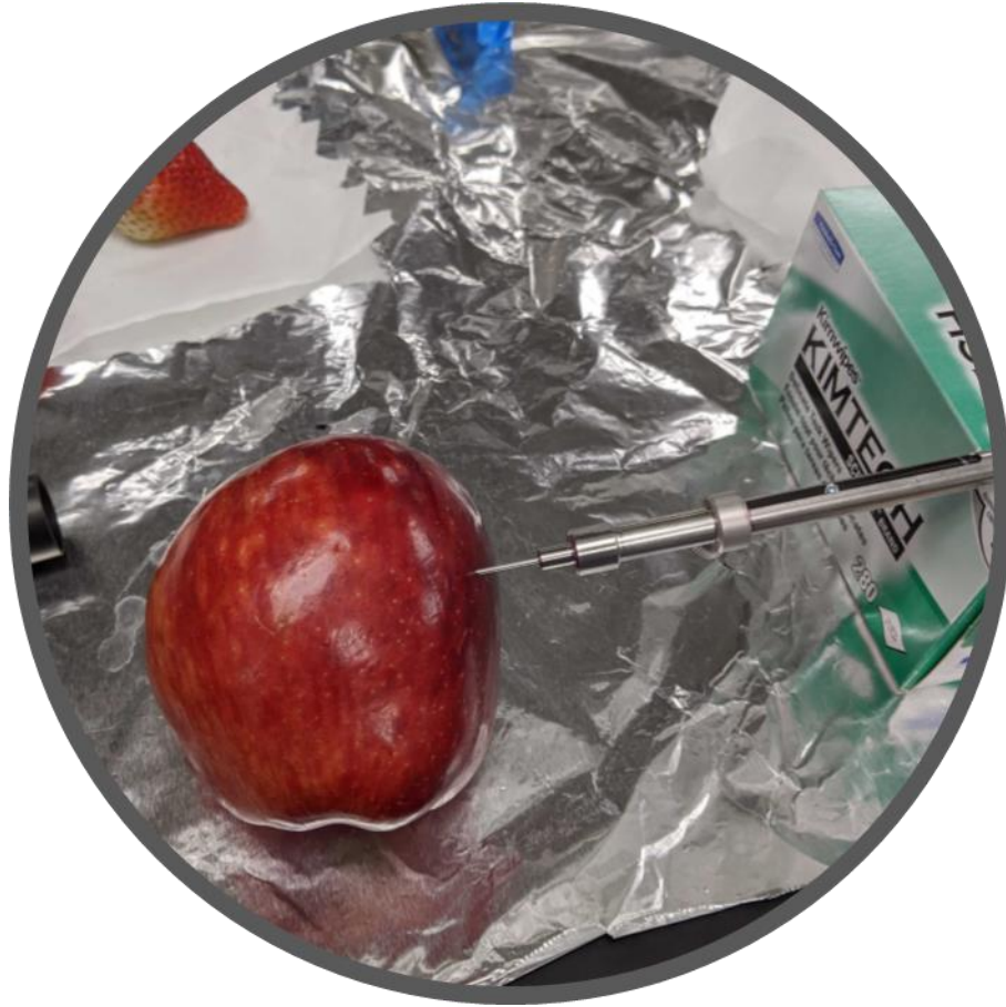
Figure 5-14 Static extraction of an apple using an SPME Arrow device.
