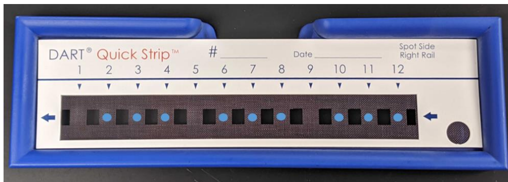
Figure 6-3 Example of sample loading on the QuickStrip, blue dots denoting sample spots with unspiked stainless-steel mesh between each triplicate.
